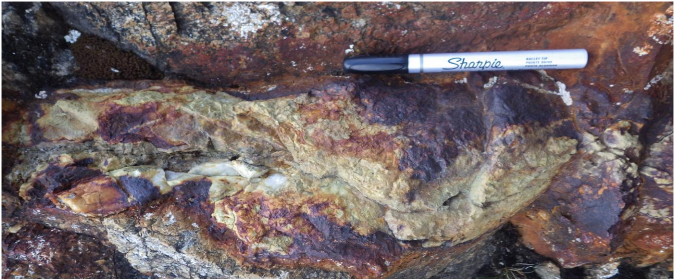
Illustration 4: Close up photo of rust bleed coming off of a discontinuous quartz vein. Yellow to white botryoidal gossan was observed to be quite prominent on some rust bleeds.
