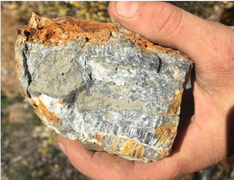
Illustration 14: Abundant fine grained pyrite within quartz vein with several generations of veining apparent
