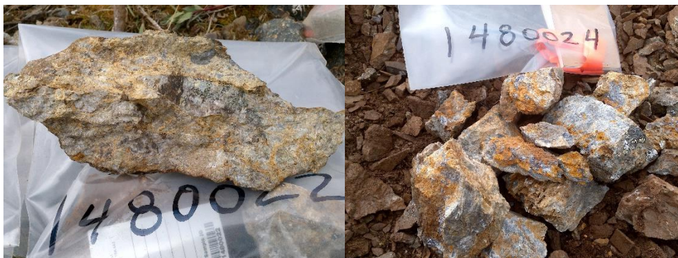
Photo Plate 3. LEFT: Unmineralized sample of the silica-healed breccia. RIGHT: Mineralized sample of the same unit
