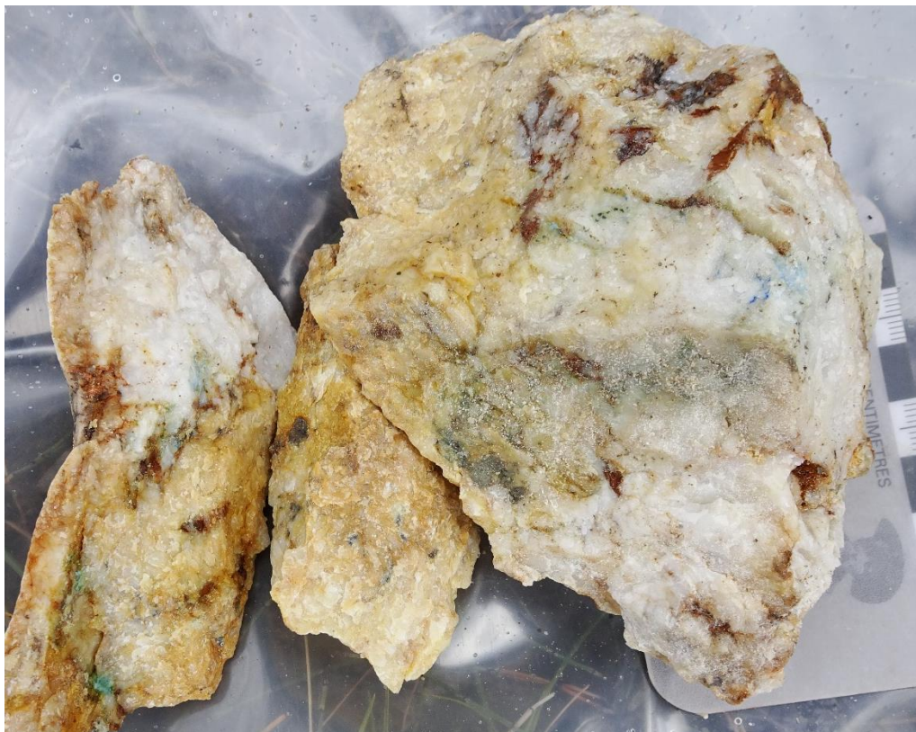
Float sample ER1952 – Grab sample from a rounded, 50x30x25 cm quartz boulder at Mars NE returned 23 g/t Au (0.67 oz/ton), with accessory copper oxides, galena and stibnite but little arsenopyrite or pyrite.
