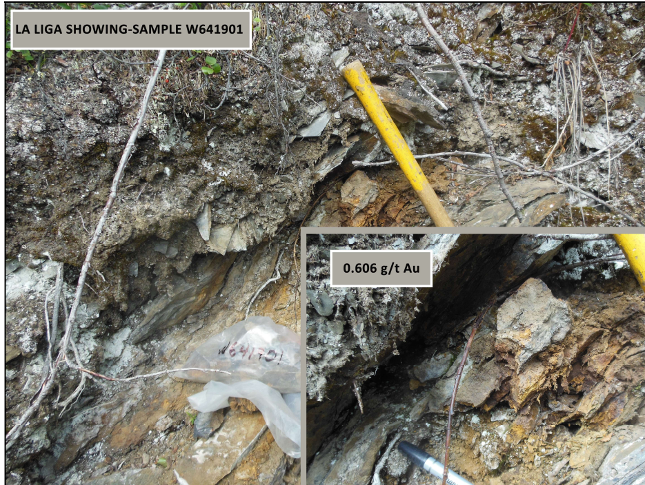
Picture 1 : Gossanous boxwork - vuggy horizon in limy shale & chip sample at La Liga showing.
