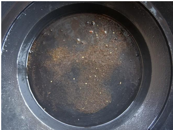
Poor recovery of very fine, flattened gold
