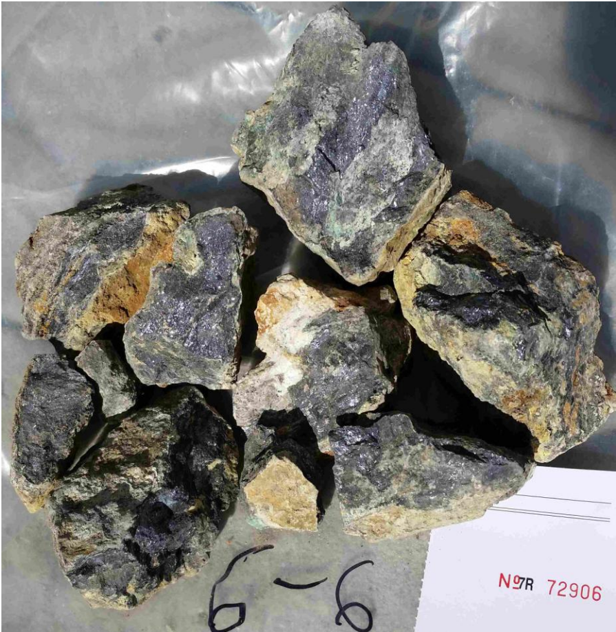
Plate 8. Sample 72906, No. 9 vein. Galena, tetrahedrite, barite. 2503 g/t Ag, 74.81% Pb.
