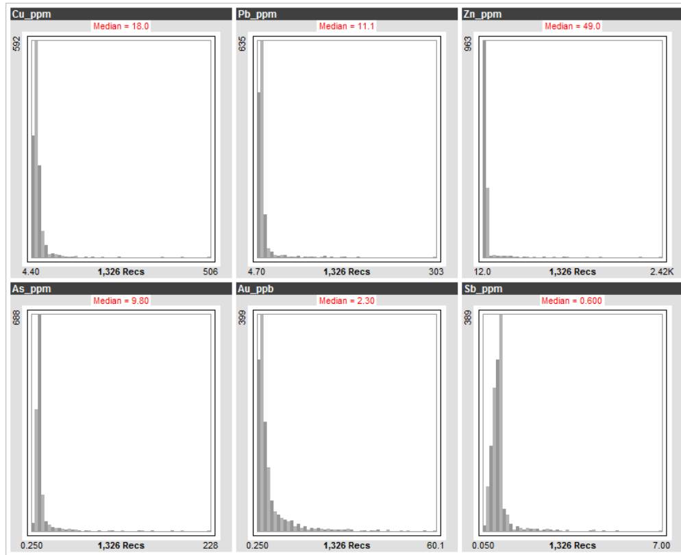
Figure 7 Histograms of Soil Samples Showing Skewed Populations for Copper, Lead, Zinc, Arsenic, Gold and Antimony.
