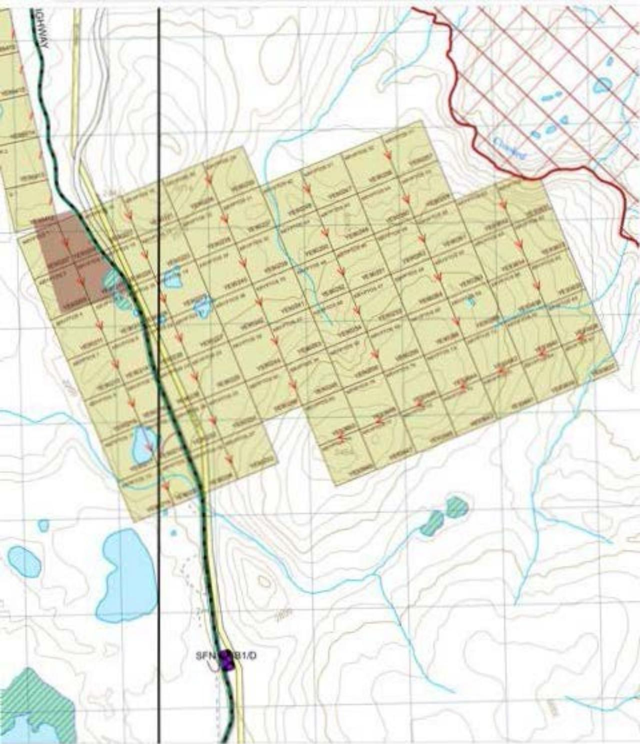
Figure 3. Local Geology of Mega Project within Kryptos Claims. Au-As-Sb-Bi-W anomalous zone was the target that was evaluated. It occurs within schists, quartzites, and phyllite of the DMF1 unit east of a northerly fault. Porphyry Cu-Au targets were not examined. See Table 2 for Legend.
