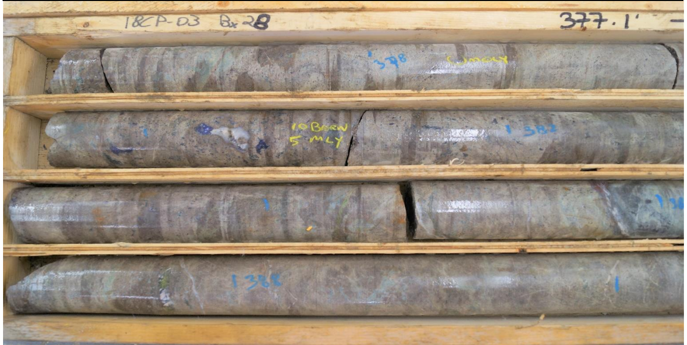
Figure 7: 18-CP-03 mineralization where 377' to 384' averaged 0.22 g/ton Au, 2.4% Cu, and 2543 ppm Mo (Samples X982779 to X982781). Garnet alteration is shown by the pervasive, light pinkish brown matrix coinciding with carbonate and diopside alteration. Bornite, chalcopyrite and molybdenite are found as semi-massive blebs withing calcite infilled hydrofracturing.
