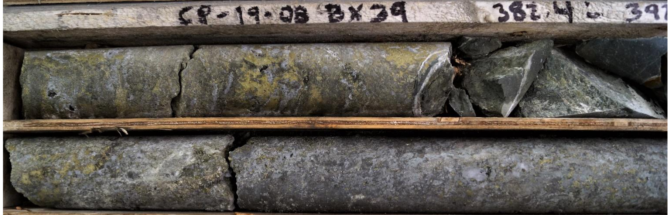
Figure 10: 19-CP-08 Mineralization; Disseminated chalcopyrite within carbonate altered magnetite skarn.
