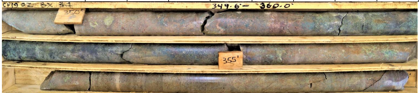
Figure 11: 19-CP-02 Mineralization; Garnet and diopside altered skarn with disseminated and fracture filling chalcopyrite, bornite, molybdenite, and pyrite. 352.4'-355.0' assayed 2.38% Cu.
