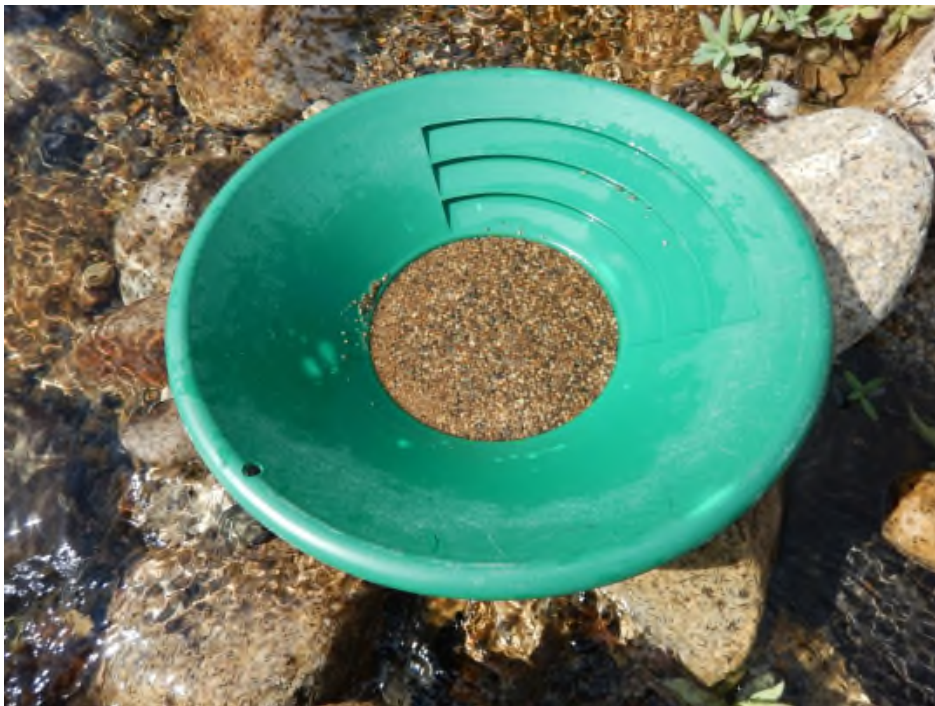
Figure 14. Photo showing stream sediment heavy mineral concentrate sample after concentration by panning (heavy mineral concentrate sample SR701; 376236E, 6665434N, UTM NAD83 Zone 9V).
