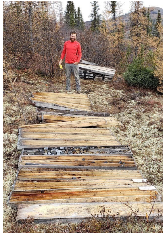
Figure 11: Hole DV07-01 core laid out on site
