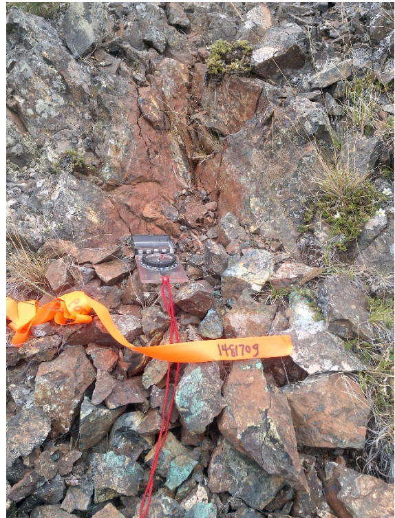
Figure 6-5: Zone D. Andesite porphyry with malachite and hematite. Sample 148709 ran 0.74% Cu and 0.406 g/t Au.
