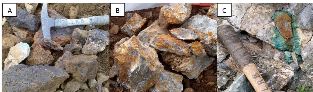
Photo Plate 4. (A) Typical alteration zones proximal to mineralization with strong to pervasive manganese and iron(-carbonate) oxides; (B) Gimli vein Ag-Pb-Zn mineralization on Nazgul claims; (C) Cu-mineralization (Saruman) on Nazgul claims as chalcopyrite nodules and malachite staining along fractures.
