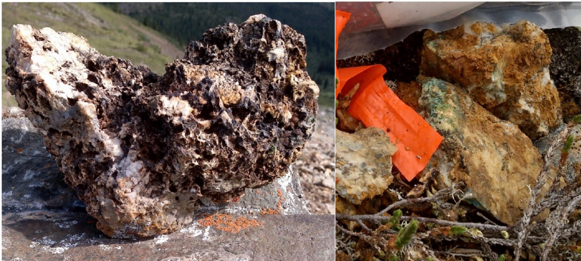
Photo Plate 5. LEFT: A sample collected from the Arkenstone vein with typical multiphase veining and copper (tenorite) mineralization infilling and replacing vugs. RIGHT: A sample collected from the intersecting Balrog structure exhibiting strong limonitic alteration.
