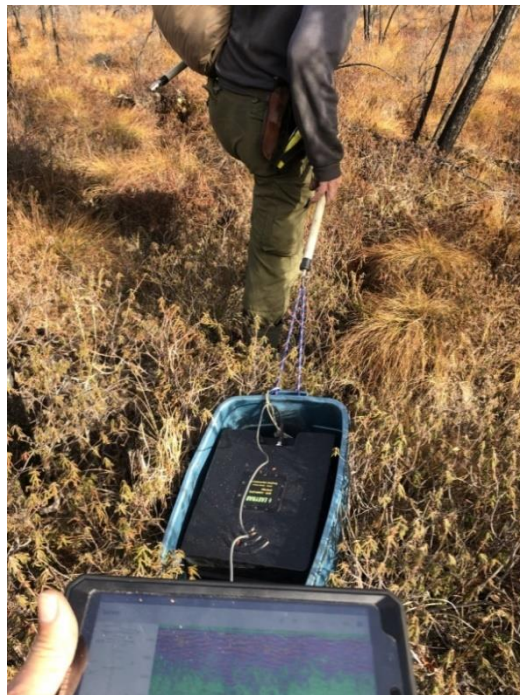
GPR-survey at Granite Gulch
