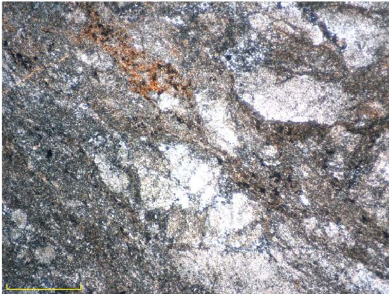
Remnant feldspars. Crossed polarizers.
