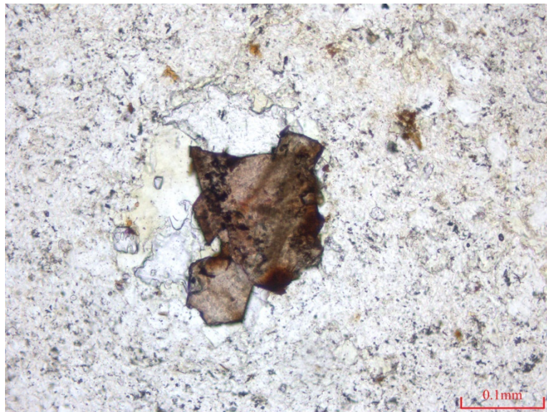
Cerite with fluorite (left, with one grain showing purple colour) and tourmaline (lower relief). P.P. light.
