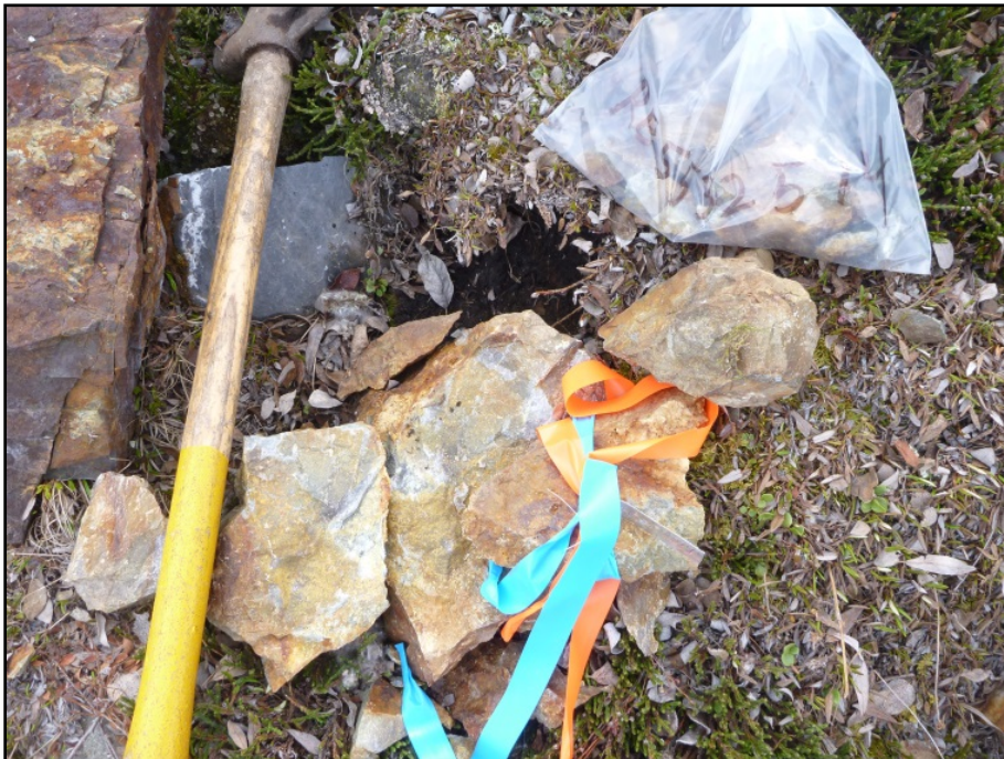
Figure 8: Sample RE5537514: Proximal float, felsic dyke returning 3.80 g/t gold
