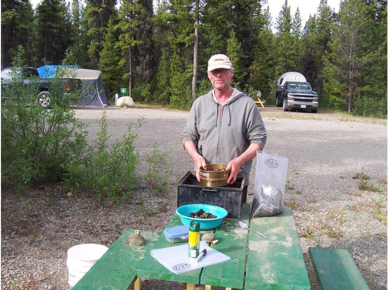
Photo 3. Author wet screening stream sediment samples to +4mm and -4mm for visual examination and laboratory analysis, respectively.
