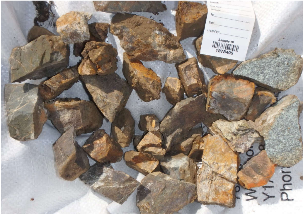
Photo 4: Sample 1878405, 8.0m – 10.0m: Oxidized and silicified quartz-sericite schist (center), sheared chloritic schist with quartz-carbonate stringers (left), and leucogabbro (right).
