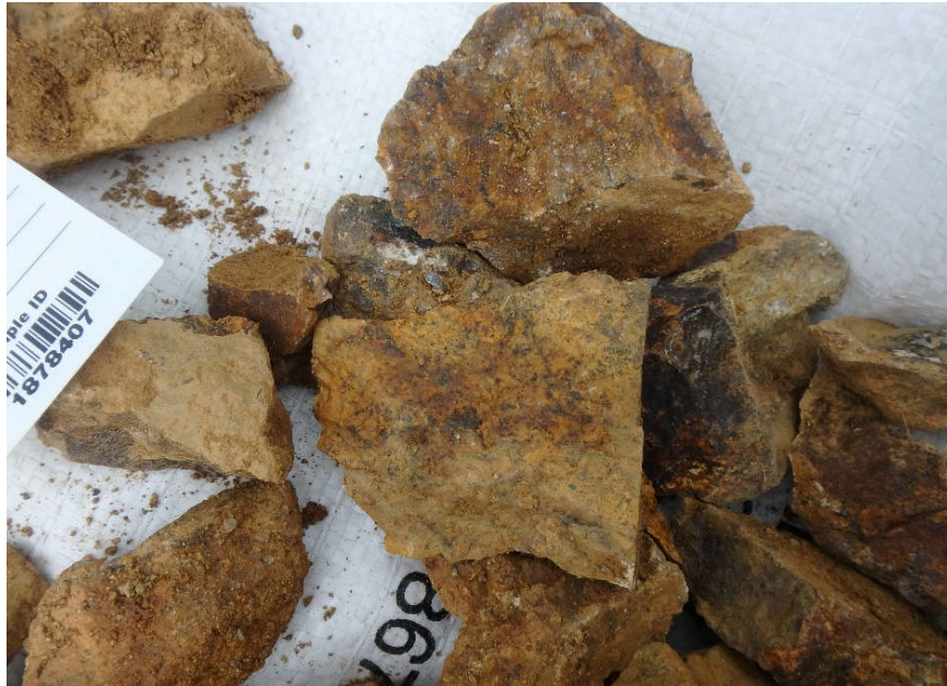
Photo 2: Sample 1878407, 12.0m – 14.0m: Oxidized quartz-sericite schist with limonitic pyrite (black spots), assaying 0.68 g/t Au over 2.0m.
