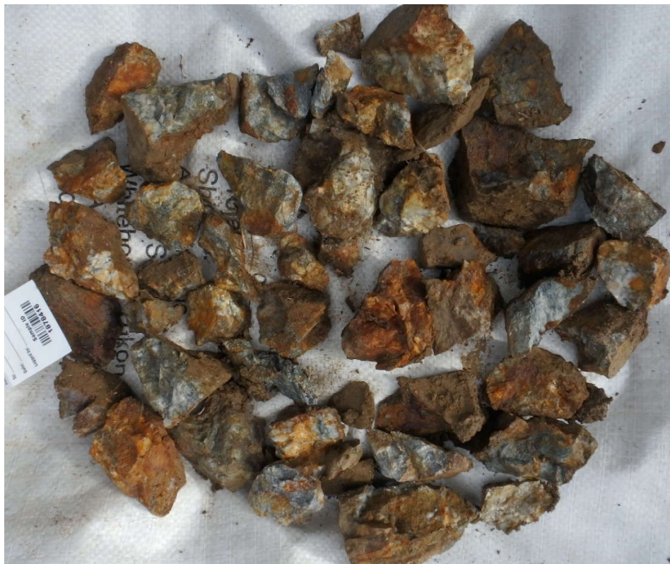
Photo 3: Sample 1878416, 30.0m – 32.0m: Oxidized and silicified quartz-sericite schist with abundant quartz stockwork, assaying 1.17 g/t Au over 2.0m.
