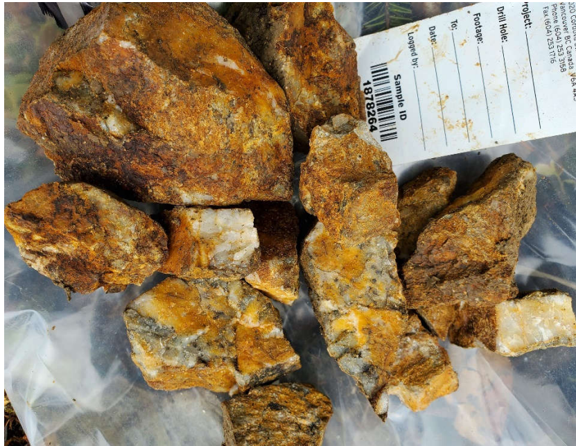
Photo 5: Pit sample 1878264 – limonitic quartz stockwork in schist with minor pyrite assayed 0.94 g/t Au
