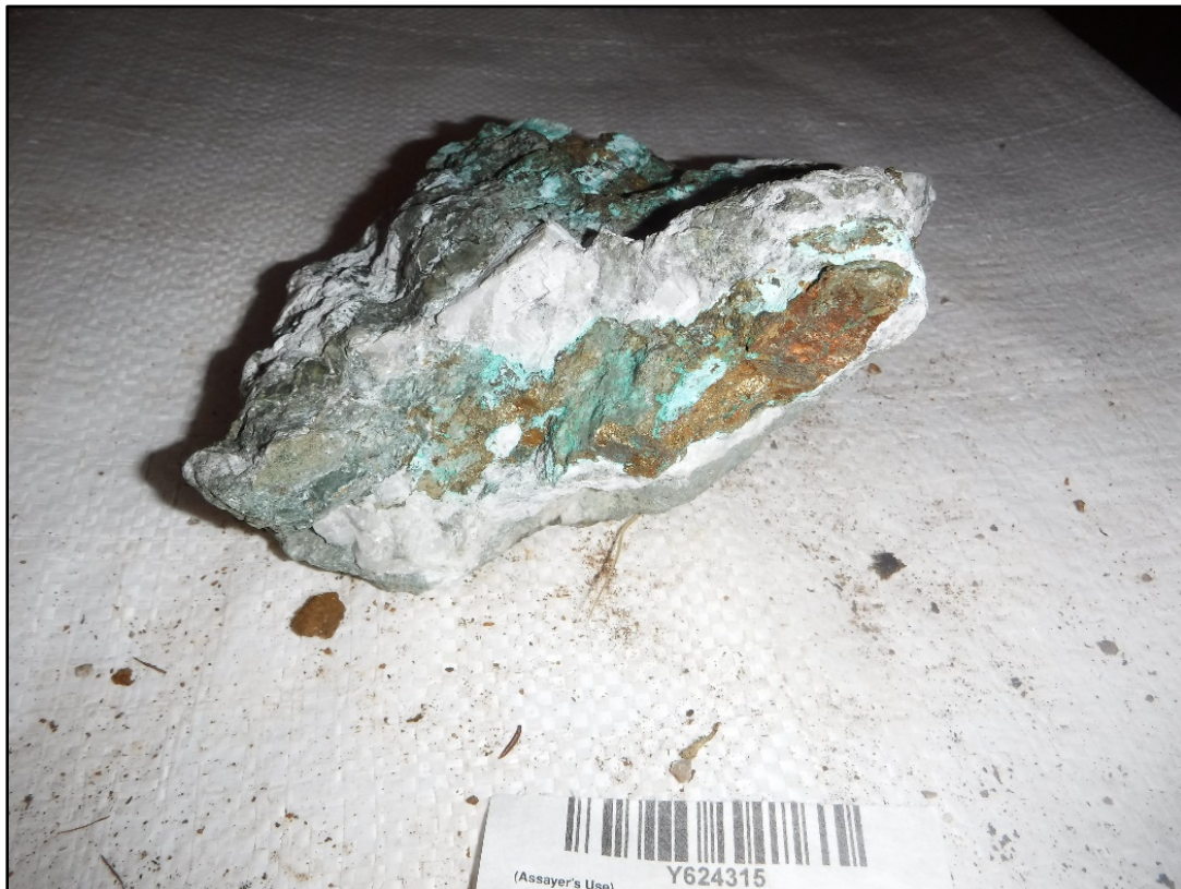
Figure 10: Banded chalcopyrite - malachite mineralization, occurrence NW of Freddy showing.
