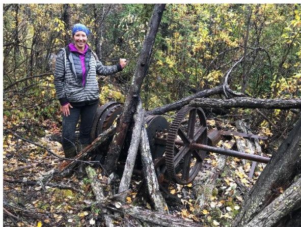
YMEP - 2020 - Found Old Timers' winch located on Max 4/ P513219, between line 07 & 08. Note this winch was powered by water wheel that runs 1000 feet of cable into the left limit old channel. Bostock writes about this portal in his Livingstone area reports.
