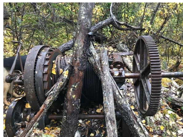
YMEP - 2020 - Found Old Timers' winch located on Max 4/ P513219, between line 07 & 08. Note this winch was powered by water wheel that runs 1000 feet of cable into the left limit old channel. Bostock writes about this portal in his Livingstone area reports.
