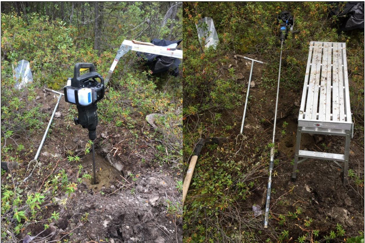
Left: Gasoline Hammer Drill at F-AD-02. Right: Gasoline Hammer Drill with sample core bit attachment (F-AD-02).
