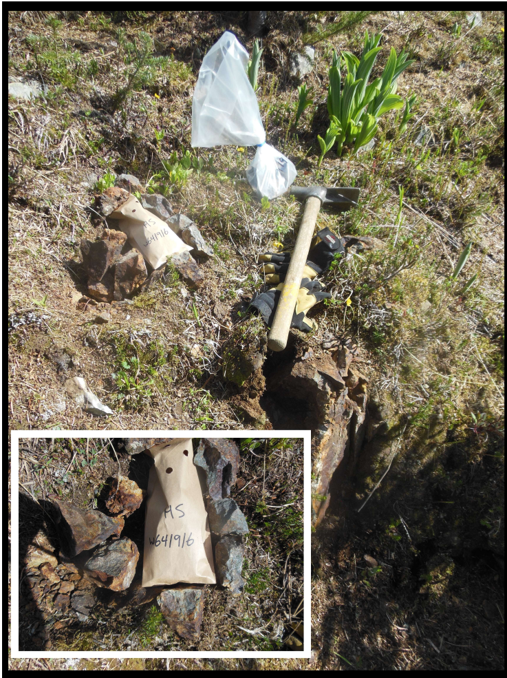
Photo 19. Sample W641916. Semi-massive sulphide float in creek bed, north of quartz-monzonite intrusion
