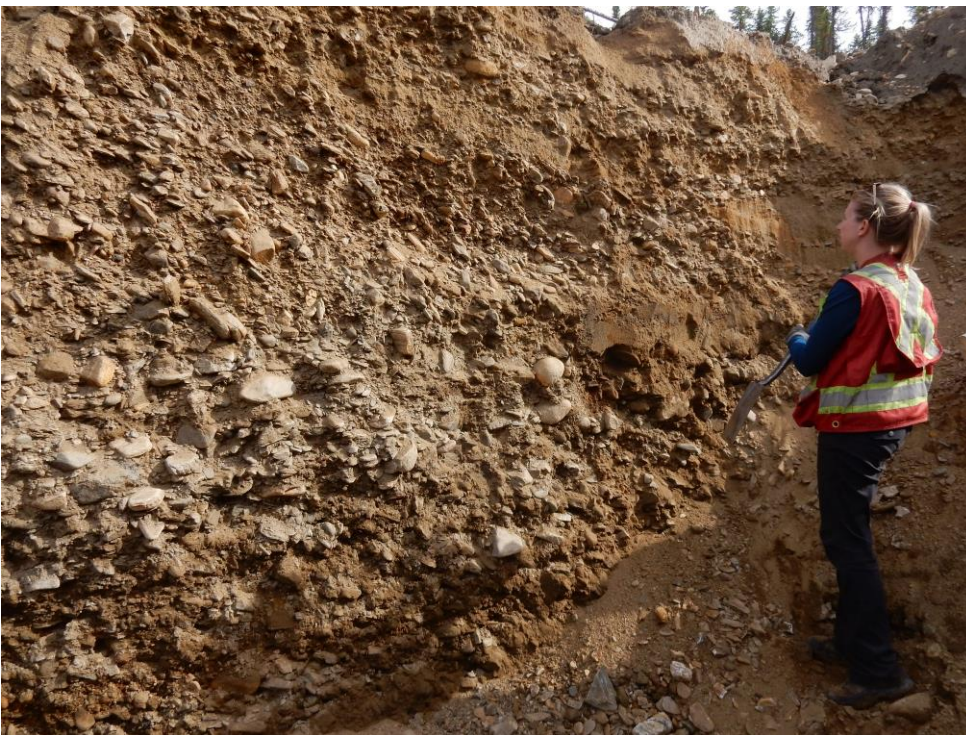
Figure 14 - Trench #3 is located downstream of Patton Creek on the right limit of Maisy May Creek, and it is approximately 5 m to bedrock. A thin muck layer was overlying the gravel, which is 4 to 5 m thick. The gravel is well-sorted and stratified with both planar tabular cross-bedding and massive channel-fill cobble-boulder groups with a sandy matrix. Two main units appear to be distinguished from each other, one has an abundance of limestone clasts and a paleoflow direction (from imbrication) which appears to trend out of Patton Creek valley, while the other has a paleoflow trend parallel to the Maisy May Creek valley.
