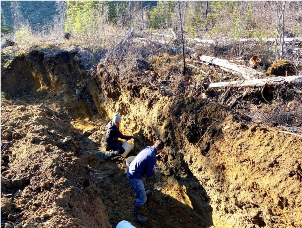
Figure 11 - Test trench #1 is located on the left limit bench of Patton Creek. This figure shows samples being collected in pails to be tested.
