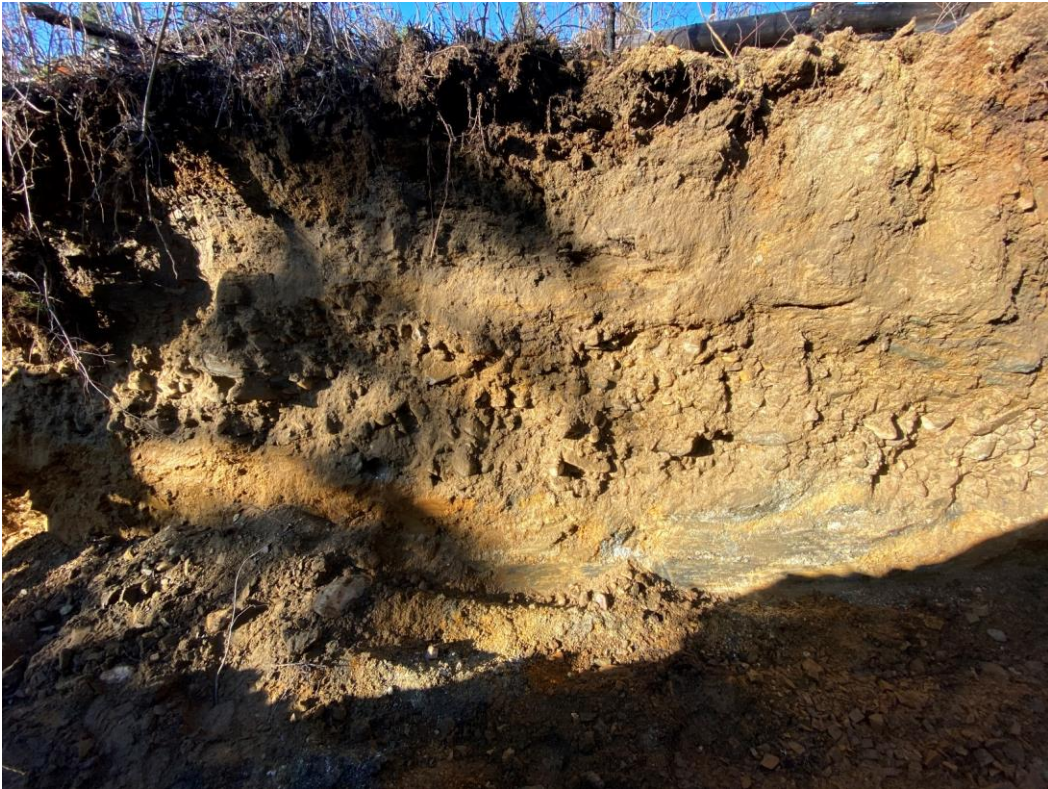
Figure 12 - Test trench #1. The total section is approximately 2 m to bedrock and displays (from ground surface) 20 cm of organics, 20 cm of tan fine sand with pebbles, 40 cm of laminated fine sand and silt. The main gravel layer is approximately 80 cm thick and consists of sub-rounded imbricated pebble-cobble-gravel with a medium to coarse sand matrix. The clasts in the gravel layer are mostly limestone with quartz and orthogneiss. The bedrock is soft, iron stained, slabby orthogneiss with some steel grey clay and silt at the bedrock contact.
