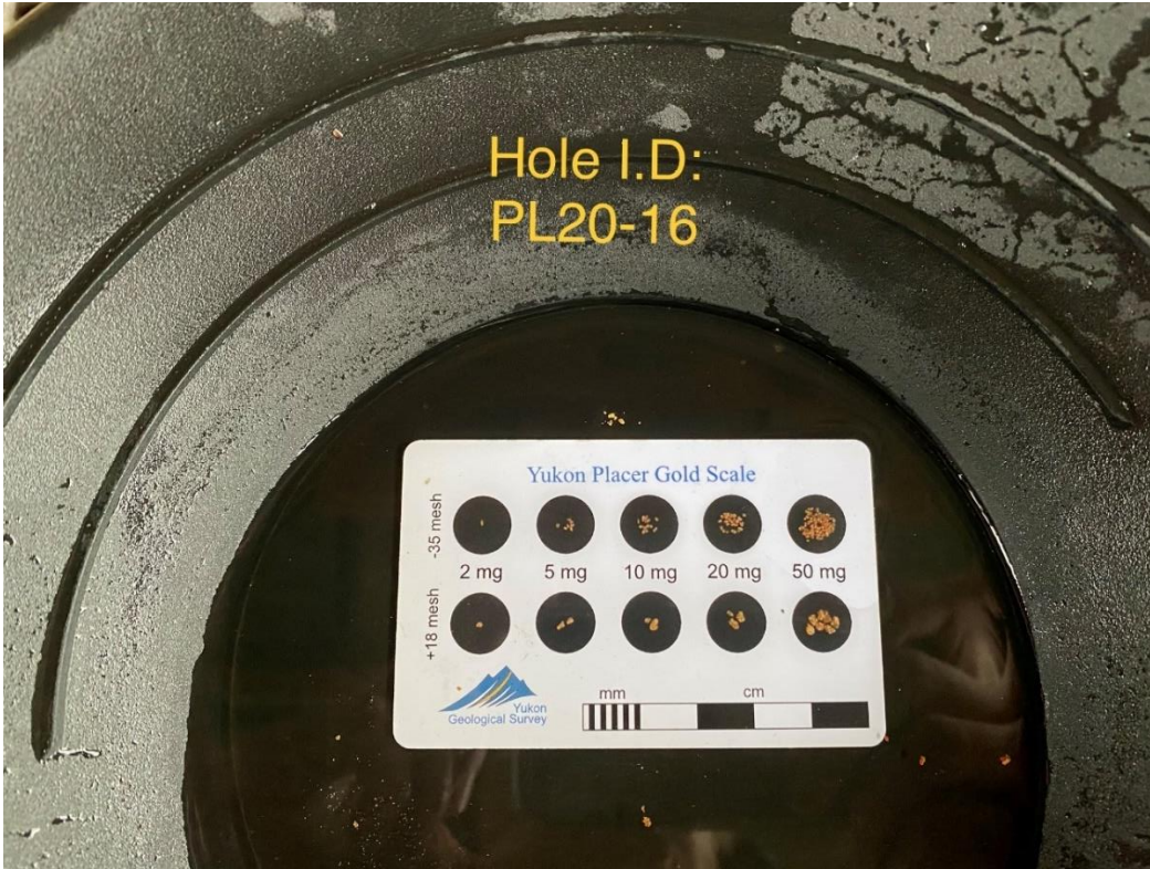
Figure 14: Gold recovered from drillhole PL20-16.
