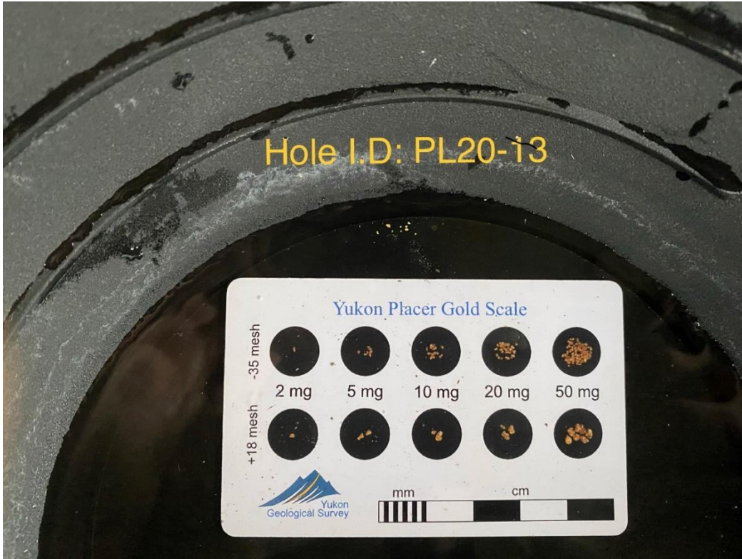
Figure 12: Gold recovered from drillhole PL20-13.
