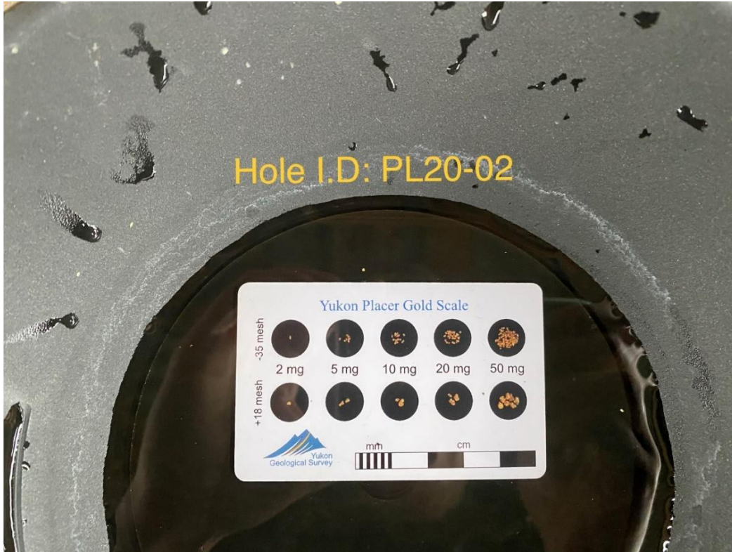
Figure 8: Gold recovered from drillhole PL20-02.
