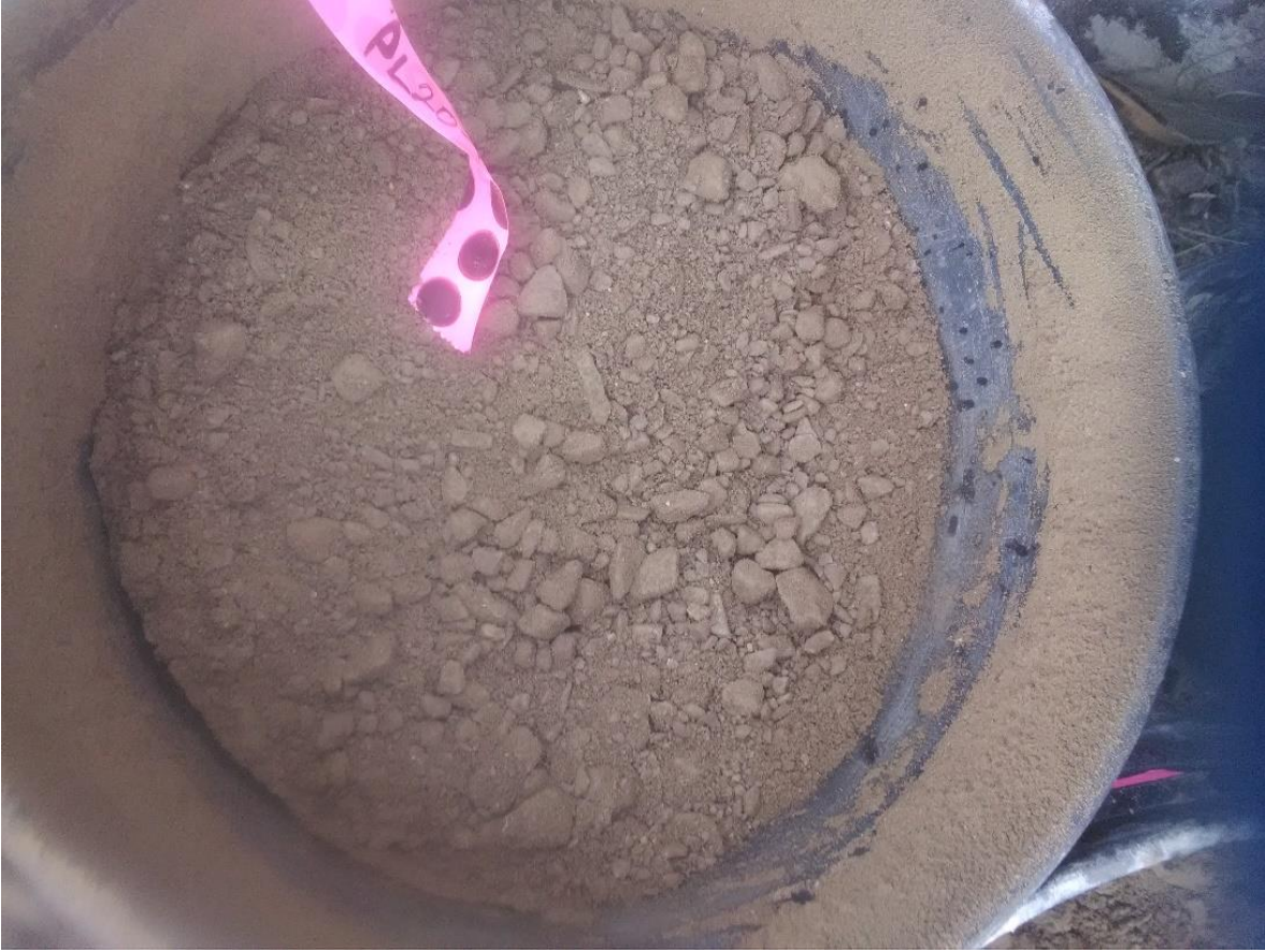
Figure 4: Bucket of return from hole PL20-12 at 25-30ft.
