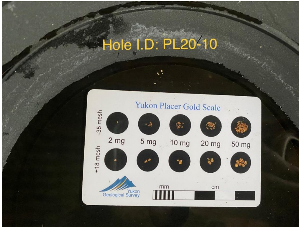
Figure 10: Gold recovered from drillhole PL20-10.
