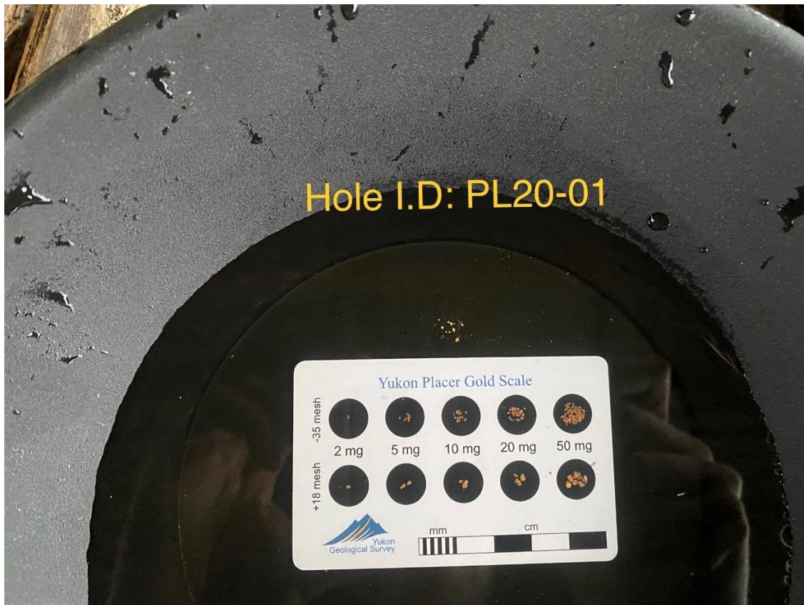
Figure 7: Gold recovered from drillhole PL20-01.
