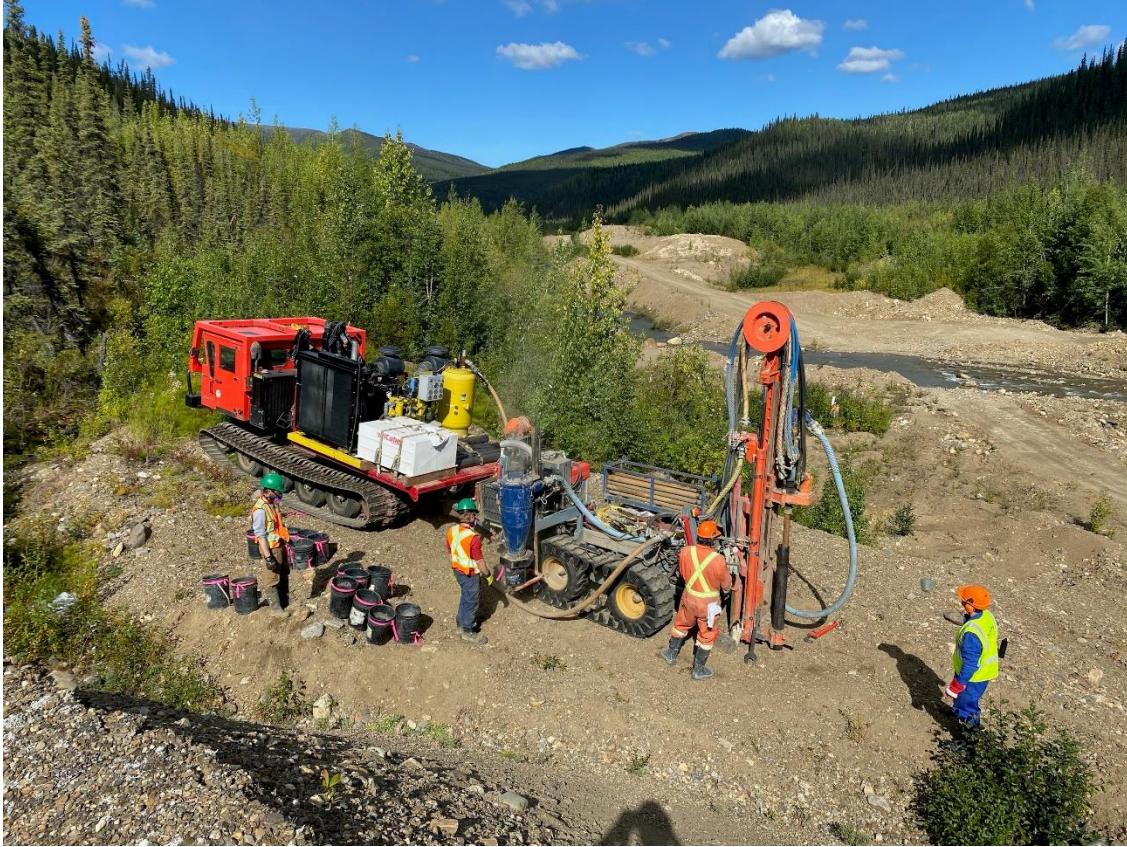
Figure 3: RC Rig set up on first drillhole of 2020.
