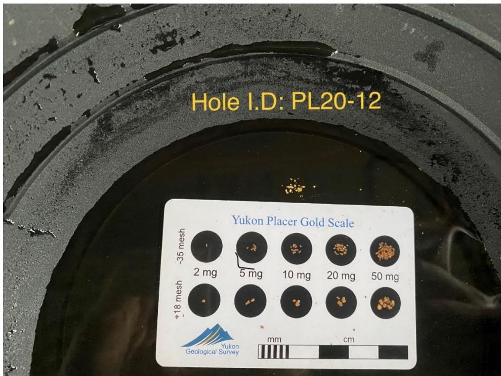
Figure 11: Gold recovered from drillhole PL20-12
