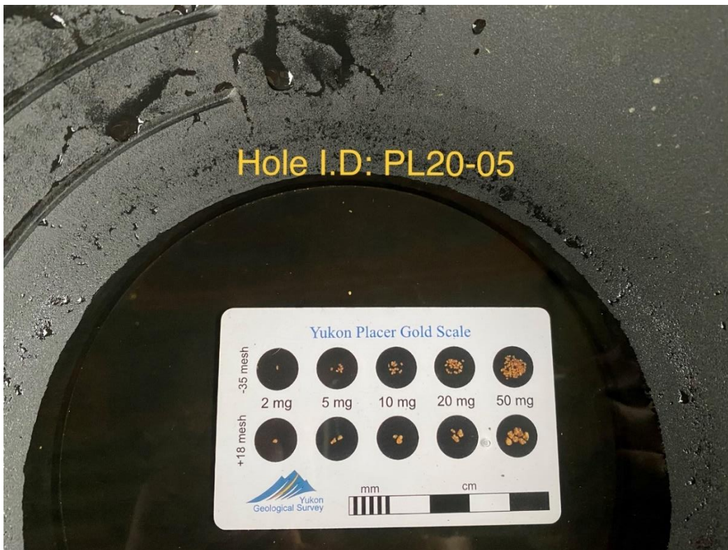
Figure 9: Gold recovered from drillhole PL20-05.
