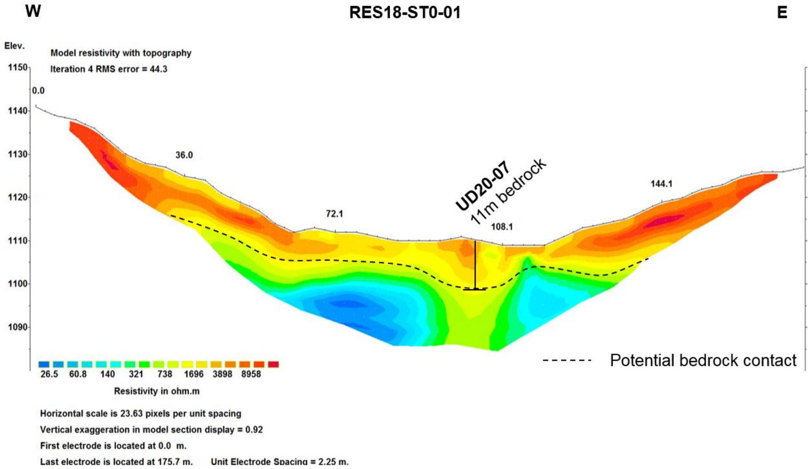
Figure 83 - RES18-ST0-01 has UD20-07 drilled on it reaching 11m with some fine placer gold from 9-11m in a gravel above bedrock.
