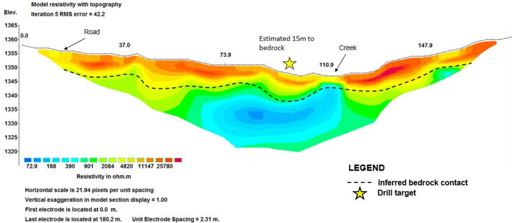
Figure 72 - RES18-JM17-01 is surveyed on the right limit of Upper Duncan Creek, on the James claims tributary. The ground in this tributary is very rocky and the high resistivity (red) displays this. In this profile, the bedrock contact is very undulatory and a drill target is identified near to the current creek.
