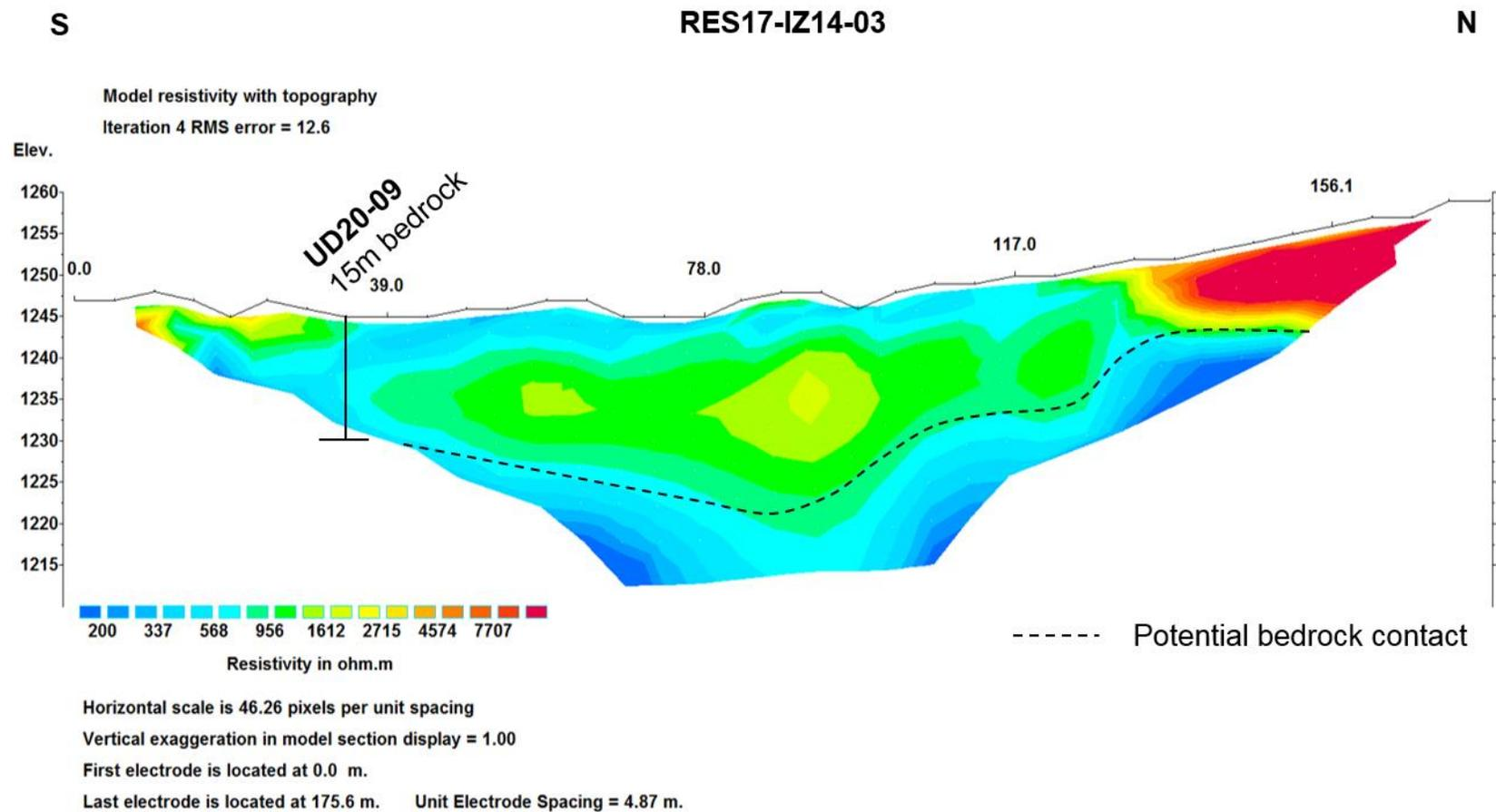
Figure 85 – RES17-IZ14-03 has UD20-09 drilled on it. The bedrock depth assists in calibrating the profile image. Fine and medium colours were found in the samples from 11-13m. Bedrock was hit at 15m.
