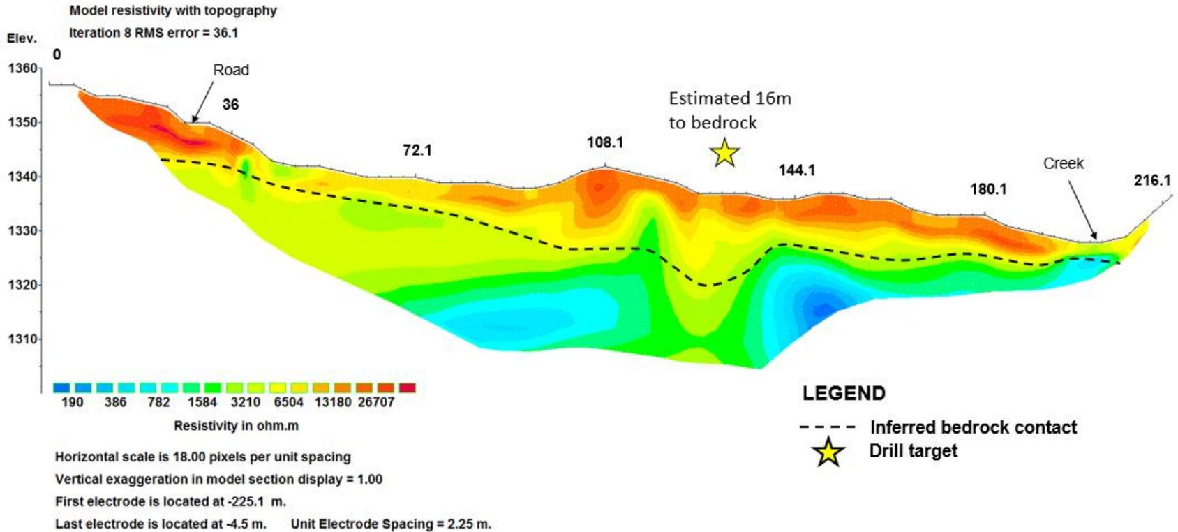
Figure 71 - RES18-JM18-01 is surveyed on the right limit of Upper Duncan Creek, on the James claims tributary. The ground in this tributary is very rocky and the high resistivity (red) displays this. In this profile, the bedrock contact is undulatory. A drill target has been chosen in the deepest interpreted bedrock.
