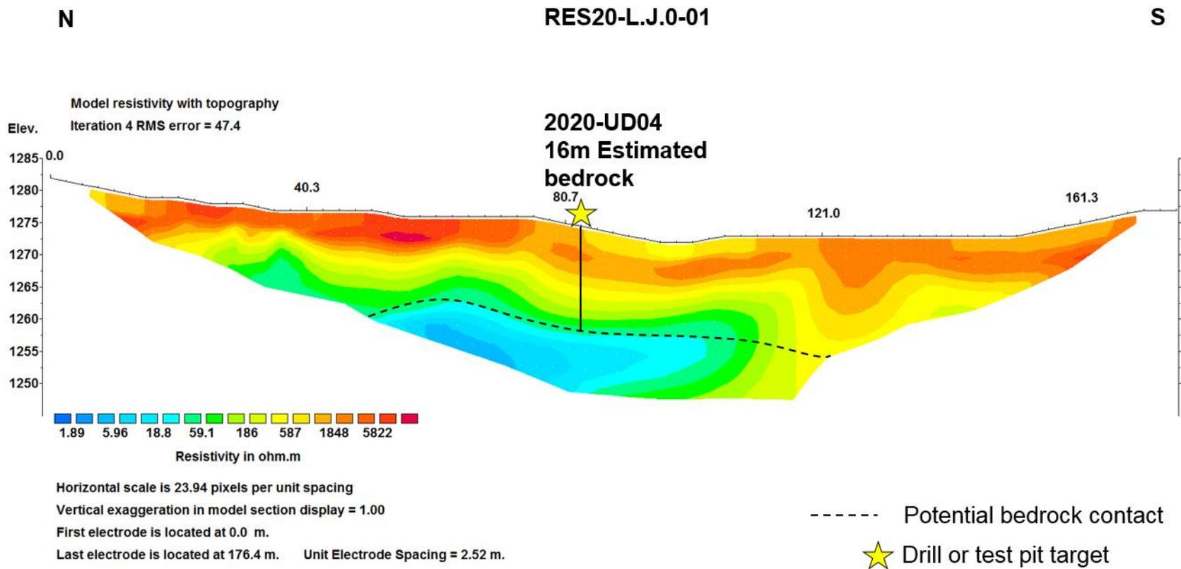
Figure 78 – RES20-L.J.0-01 is surveyed from north to south. The survey is viewed looking upstream in the Lindsey claim area. The bedrock contact is interpreted slightly undulating with 1 target picked on the right limit of the creek. The interpreted depth is 16m and the expected stratigraphy is colluvium overlying reworked Reid aged till on bedrock which could be a host to placer gold.
