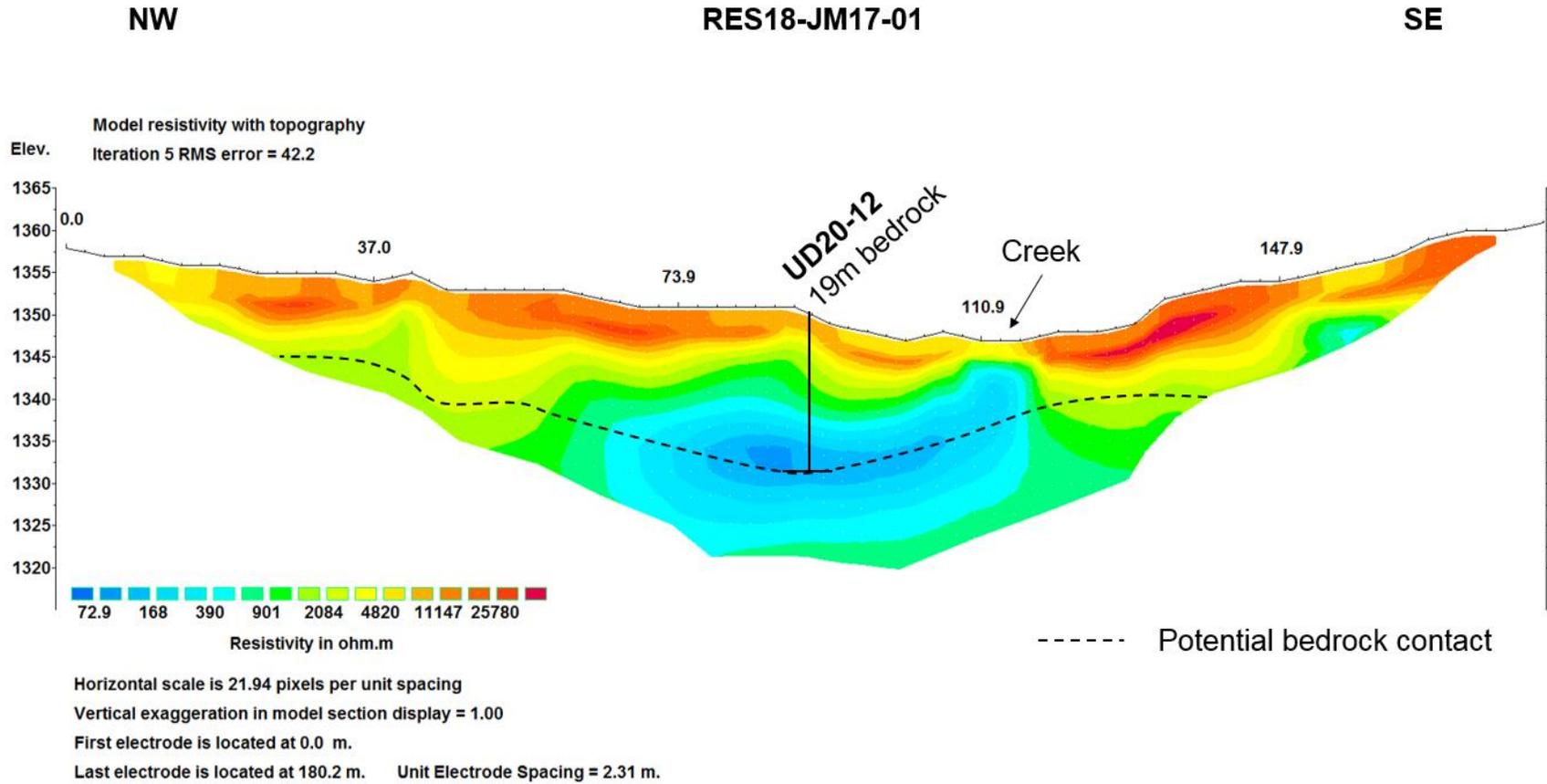
Figure 87 - RES18-JM17-01 has drill hole UD20-12 drilled on it. The drill hole had no gold in it. The material drilled is interpreted as McConnell age till.
