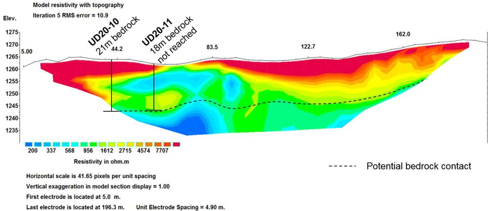
Figure 86 – RES17-IZ14-01 has 2 drill holes (UD20-10 and UD20-11) drilled on it. The bedrock was reached at 21m in UD20-10 and was not reached due to drill problems and excess water pressure while drilling. UD20-10 has good gold content from 16m-22m, the layer above bedrock. The gold was found in a brown sandy gravel overlaid by a black gravel with silt.
