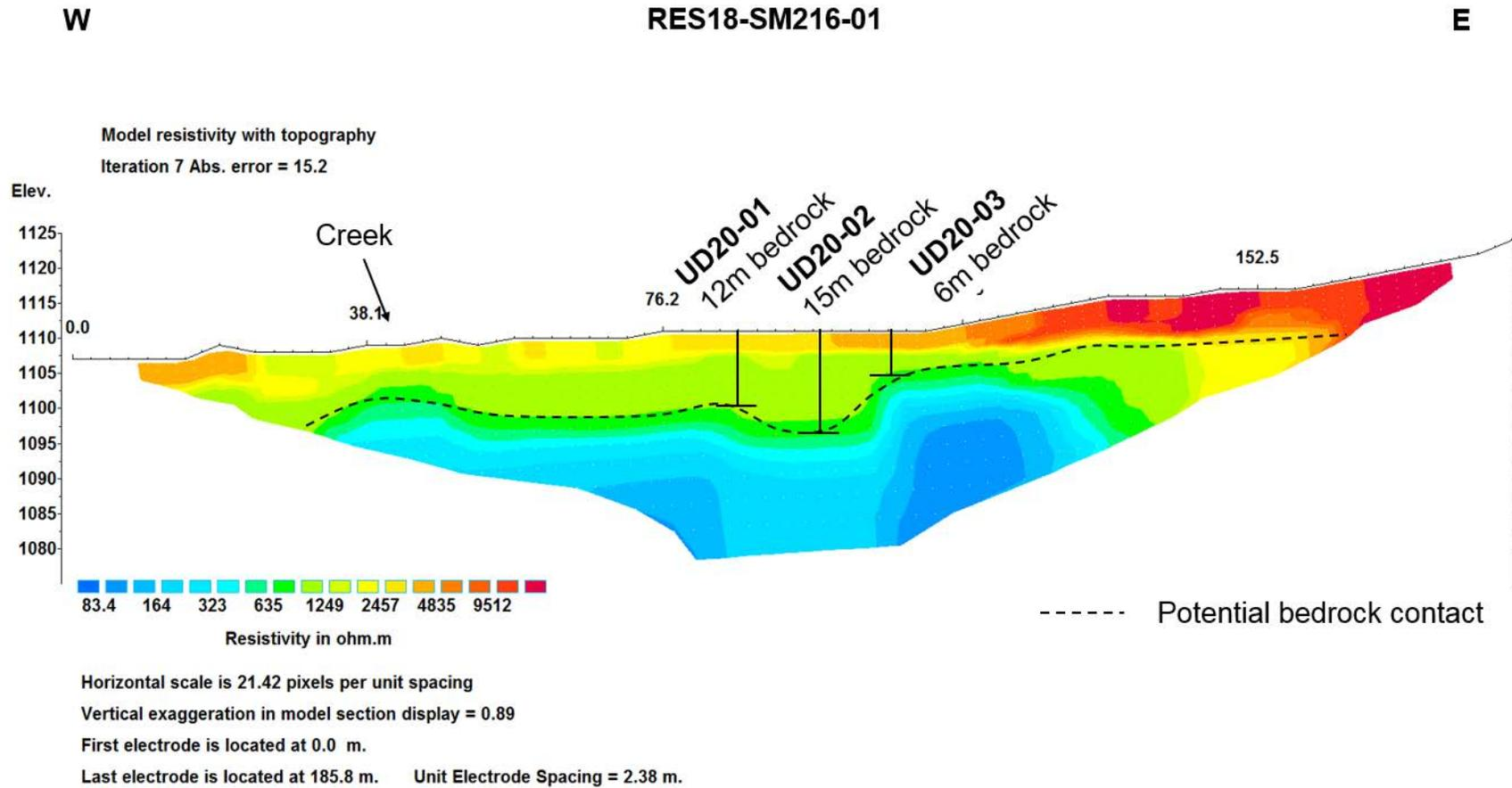
Figure 81 – RES18-SM216-01 had a target that was drilled in 2020 with UD20-01, 02 and 03. The respective depths reached are 12m, 15m, and 6m. UD20-01 yielded the best placer gold results with a 4m zone of gold content. The bedrock depth correlated nicely with the projected target bedrock depth.
