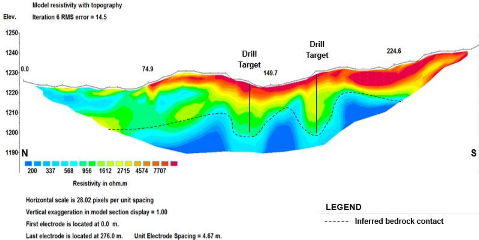
Figure 37 - RES17-IZ12-01 was surveyed across a moraine and appears to display large undulations in the bedrock contact. The large undulations are drilling targets for depth calibration and to examine possible gold values.
