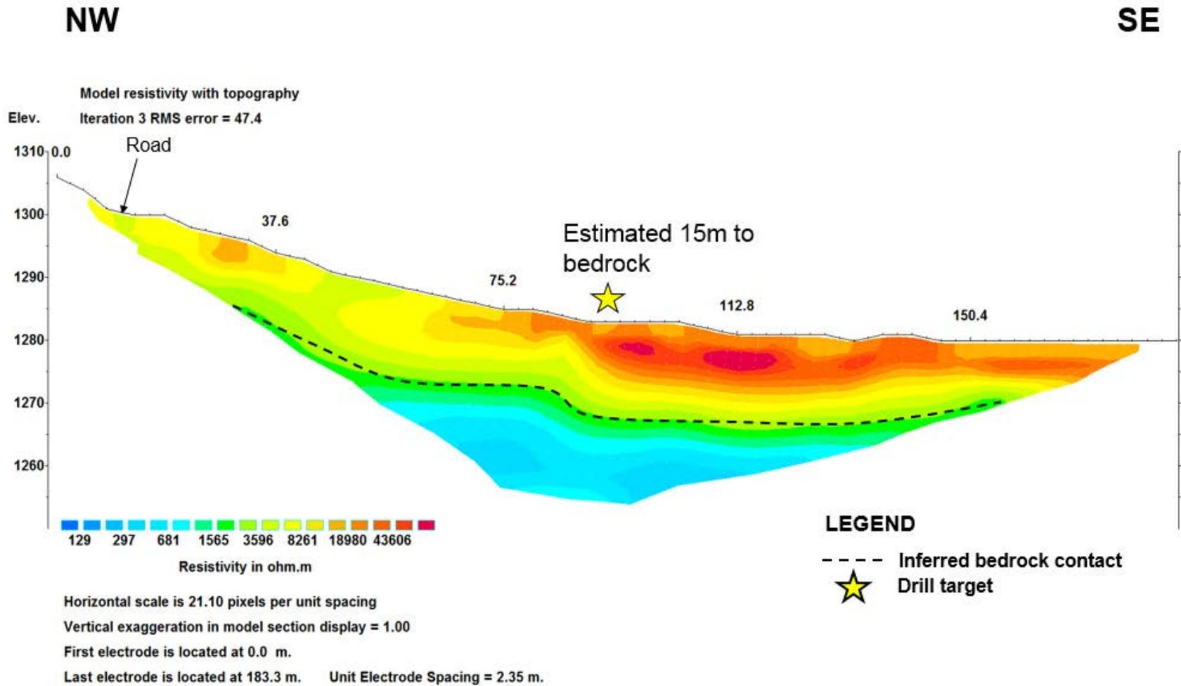
Figure 68 - RES18-LEW3-01 is located on the right limit of Upper Duncan Creek. The ground in this narrow gulch-like valley is very rock, which shows as high resistivity values (red) on the surface. A slightly undulating bedrock contact is interpreted with a drill target identified in the deepest undulation.
