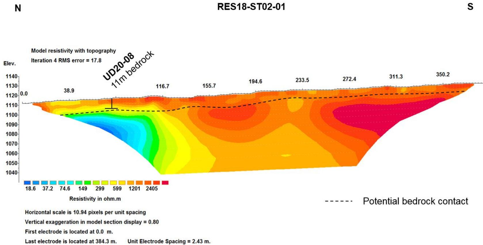
Figure 84 - RES18-ST02-01 has drill hole UD20-08 on it. There were no gold values found in this drill hole, however, the bedrock depth calibrates the geophysics.
