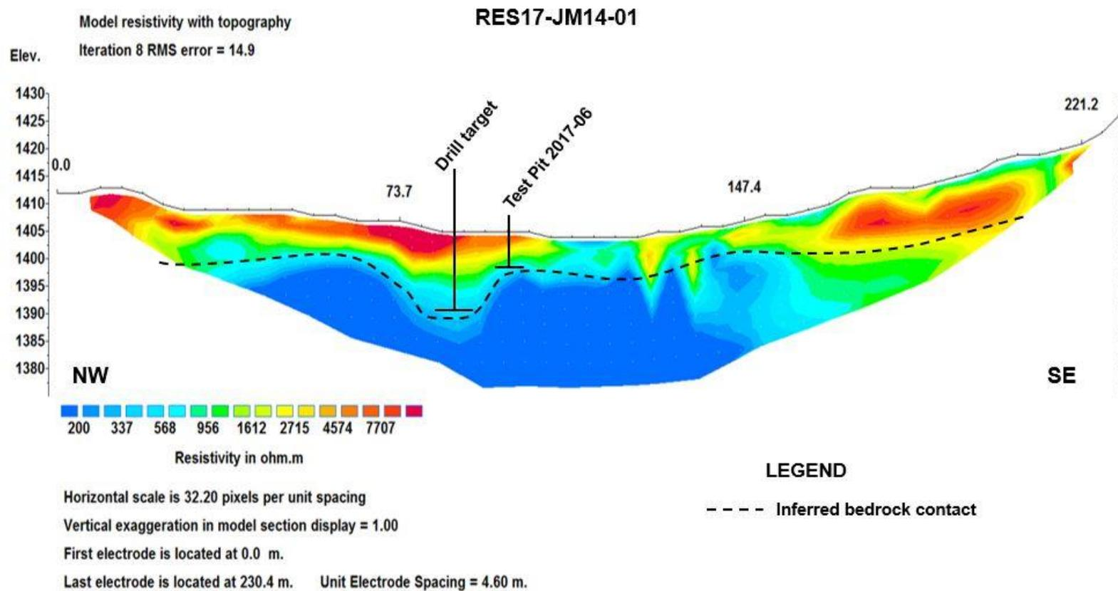
Figure 13 - RES17-JM14-01 is downstream of RES17-JM11-01. This profile has an interpreted bedrock contact that gently undulates except for a bedrock depression, which is a proposed drill target at 85 metres. Test Pit 2017-06 appears to have reached bedrock at approximately 7 m in a location adjacent to the bedrock depression.
