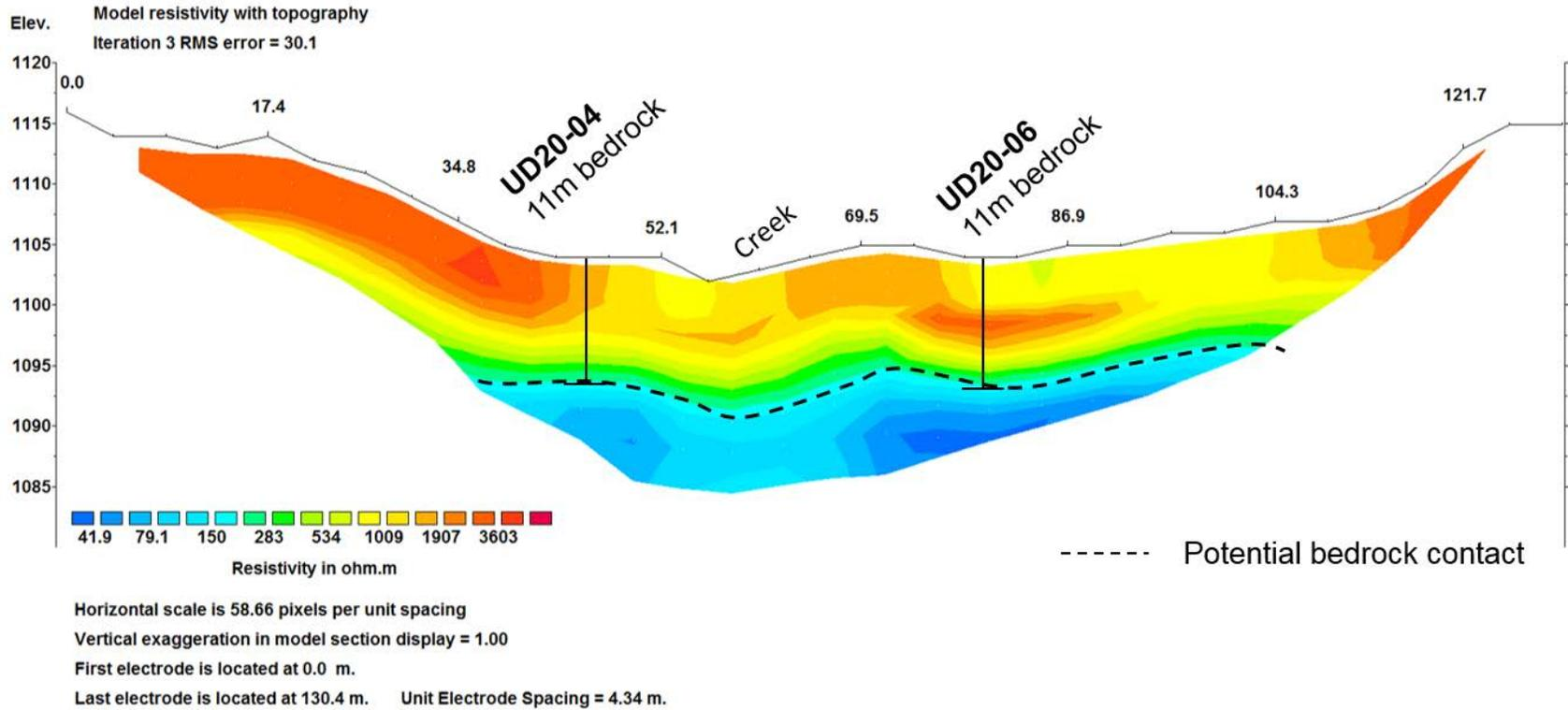
Figure 82 -RES17-SM216-01 had 2 drill holes (UD20-04 and UD20-06) along the survey line, with UD20-05 being drilled just 10m south of UD20-04. Drill holes UD20-04 and 06 both had fine colours in the gravel just above bedrock.
