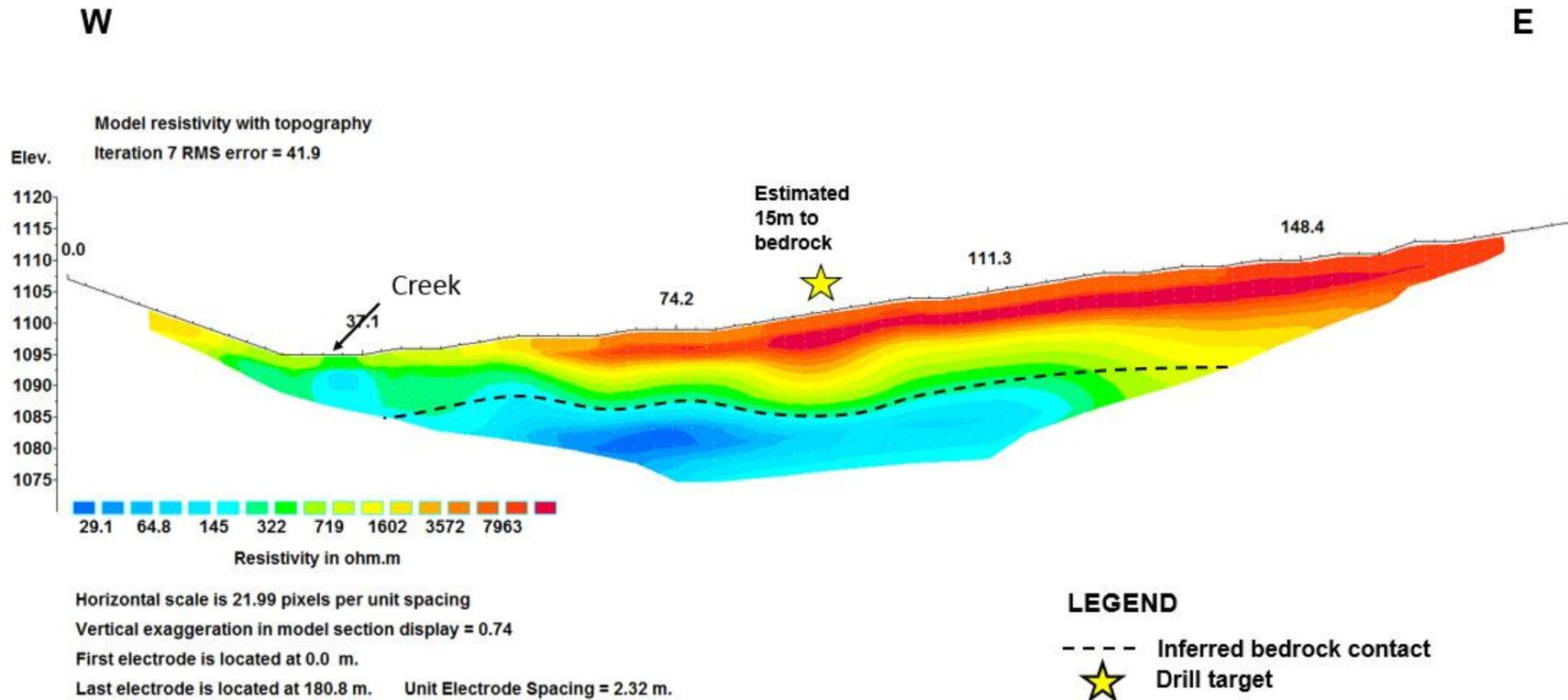
Figure 55 - RES18-JL2-01 is surveyed across the mouth of the Jill tributary. The interpreted bedrock profile shows a undulation on the right limit bench that could host placer gold. This bedrock undulation has been identified as a future drill target.
