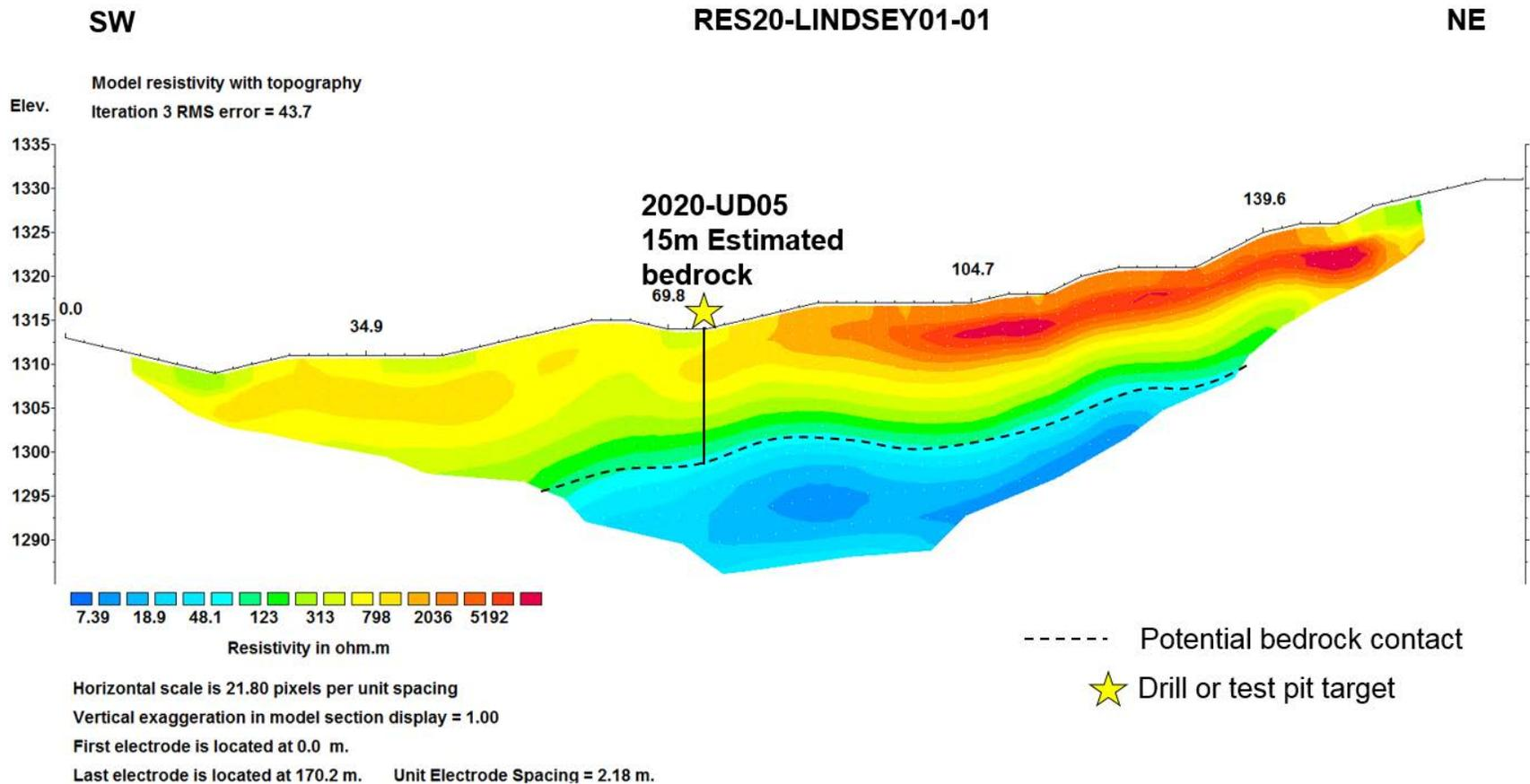
Figure 79 - RES20-LINDSEY01-01 is surveyed from southwest to northeast. The survey is viewed looking downstream in the Lindsey claim area. The bedrock contact is interpreted slightly undulating with 1 target picked on the right limit of the creek. The interpreted depth is 15m and the expected stratigraphy is colluvium overlying reworked Reid aged till on bedrock which could be a host to placer gold.
