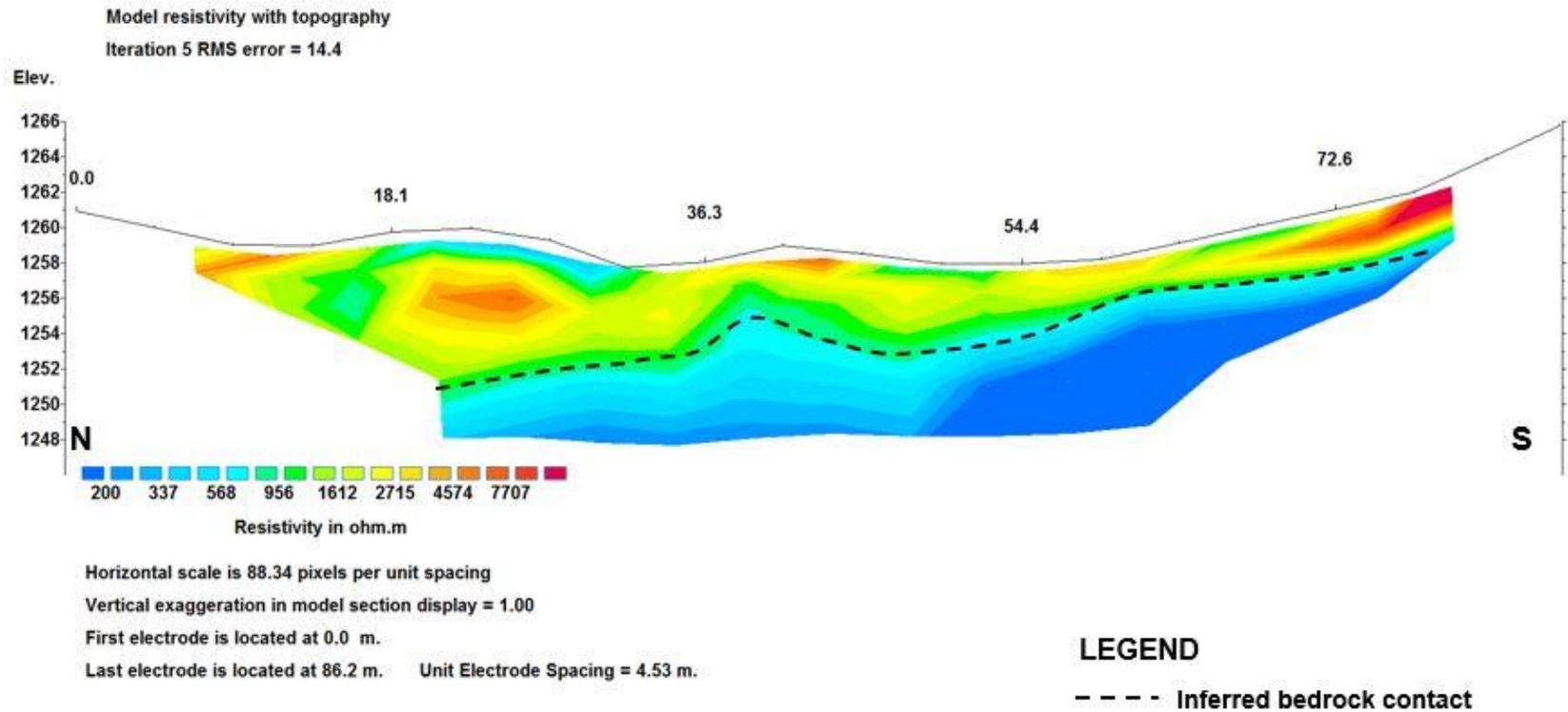
Figure 19 - RES17-IZ15-01 was surveyed across the main Izzie test pit. Bedrock was distinctive as well as the possible left limit bedrock bench seen on other profiles.
