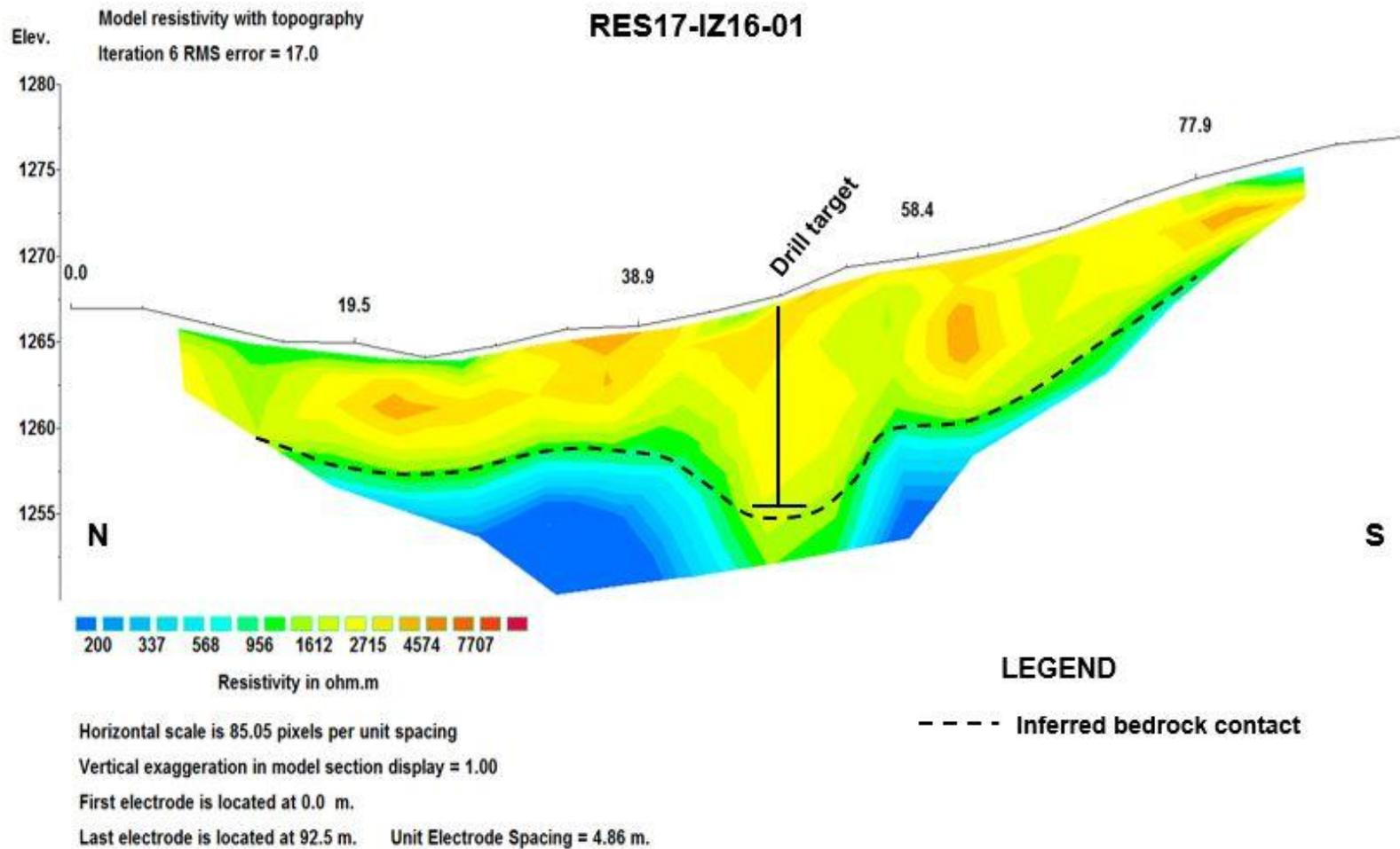
Figure 17 - RES17-IZ16-01 is located upstream of the excavated test pit and exhibits a narrow depression and a zone of high resistivity in the centre. A drill target is proposed.
