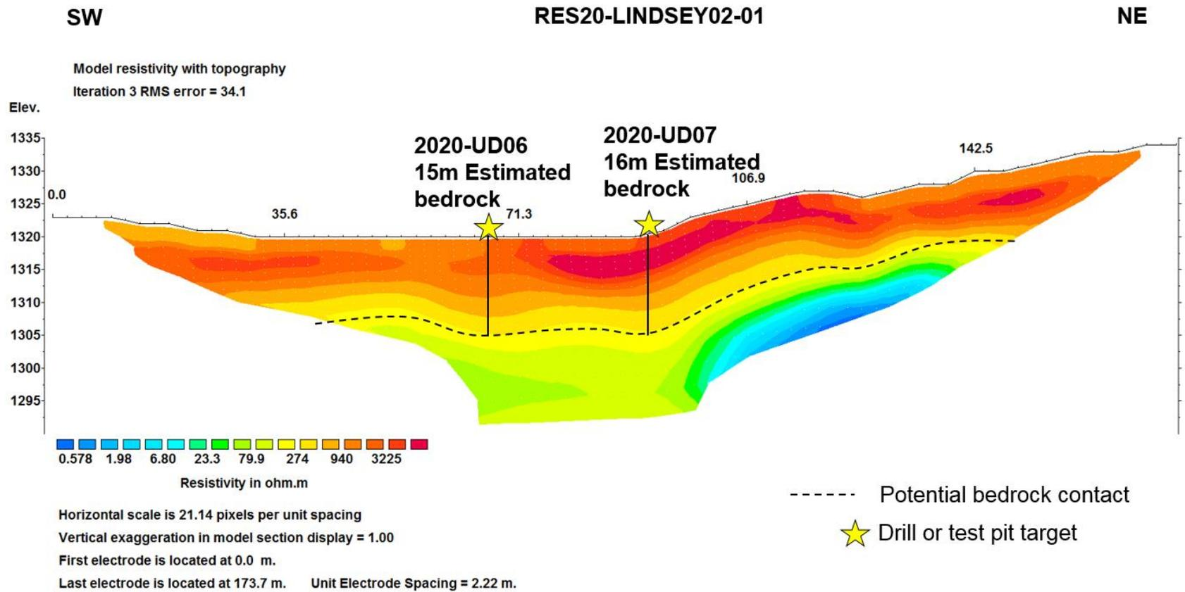
Figure 80 -RES20-LINDSEY02-01 is surveyed from southwest to northeast. The survey is viewed looking downstream in the Lindsey claim area. The bedrock contact is interpreted slightly undulating with 2 targets picked on the right limit of the creek in a flat topographical area. The interpreted depths are 15m and 16m and the expected stratigraphy is colluvium overlying reworked Reid aged till on bedrock which could be a host to placer gold.
