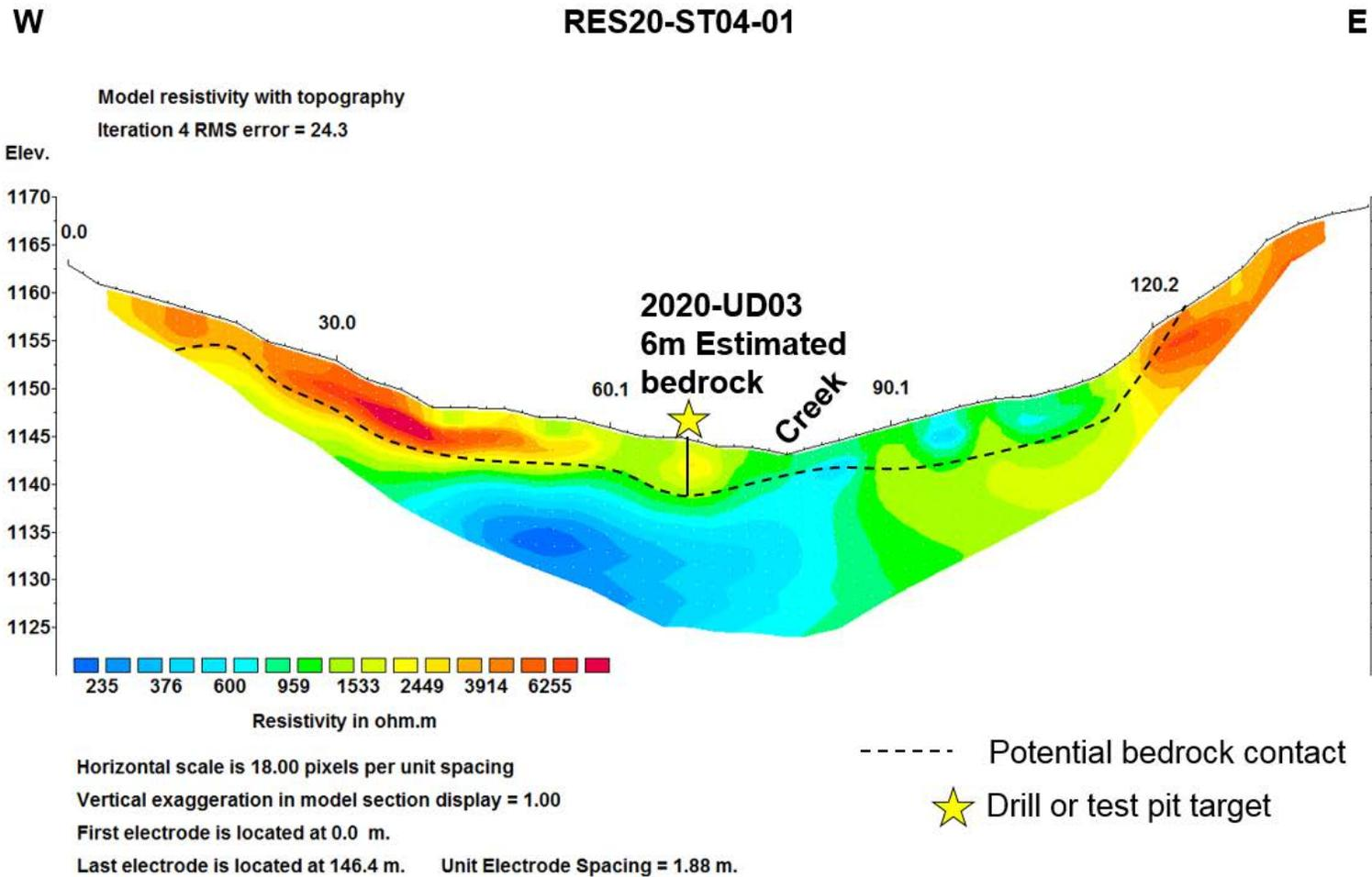
Figure 77 – RES20-ST04-01 is surveyed from west to east in the Stuart claims tributary of Upper Duncan Creek. The profile is viewed looking downstream. The bedrock profile interpreted has a slightly undulating surface and there is 1 drill target chosen in the deepest undulation with depth of 6m. The expected surficial units encountered in the targets would be colluvium overlying paleochannels of reworked till.
