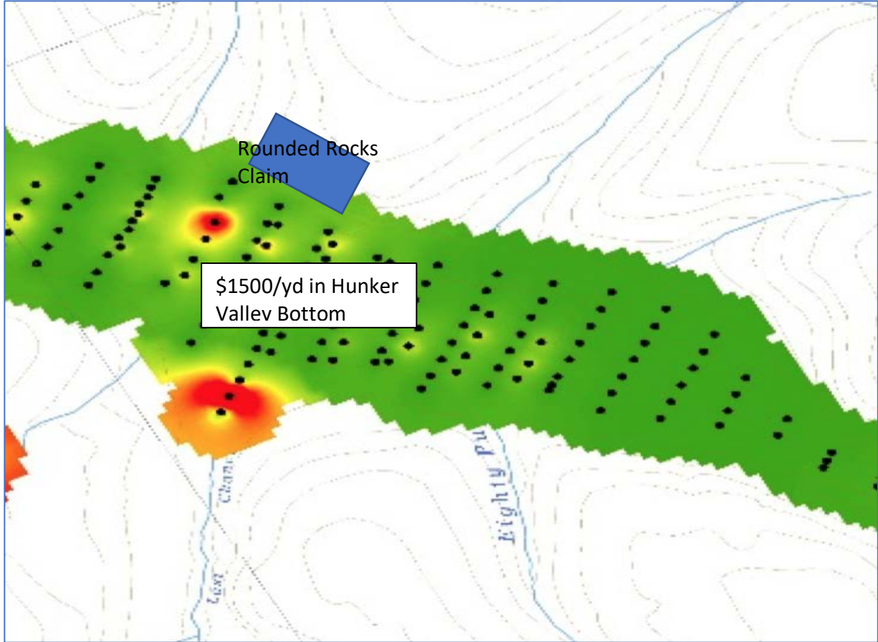
Figure 11. Detail of map above showing extremely high gold grades that were identified by YCGC drilling directly downhill of the Rounded Rocks claim
