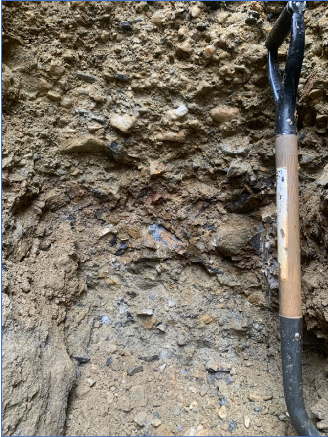
Figure 17. Section showing transition between clast-matrix (top) and sand matrix (lower) that correspond to the first (erosional) and second (aggradational) phases of White Channel deposition at the joint of the shovel blade and metal handle. This is superseded by an organic-rich mud lacustrine layer 1-2 m thick (third phase) and is capped by a 1m thick layer of sand and gravel (fourth phase) as per (Lowther et al, 2014)'s model.
