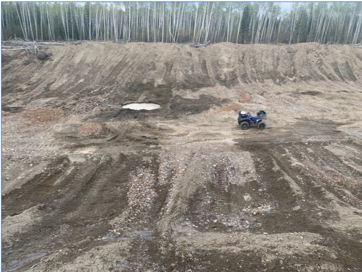
Figure 3. Test pit filled with groundwater. Area of investigation prior to significant bulk sampling. Note red-coloured gravel patches. These contained significantly more and coarser gold than the surrounding grey gravels.
