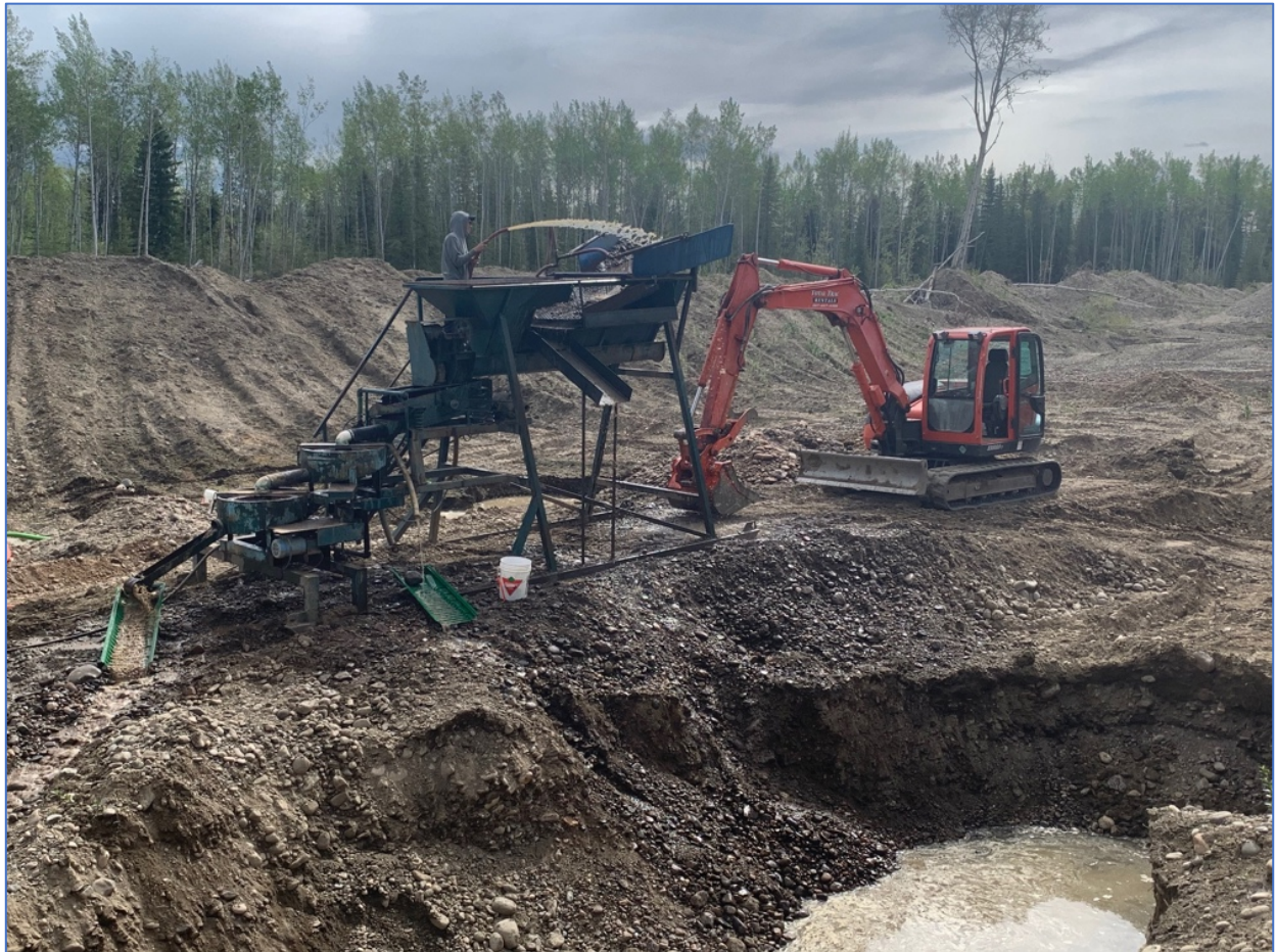
Figure 4. Test pitting with centrifugal plant and Kubota 080 excavator
