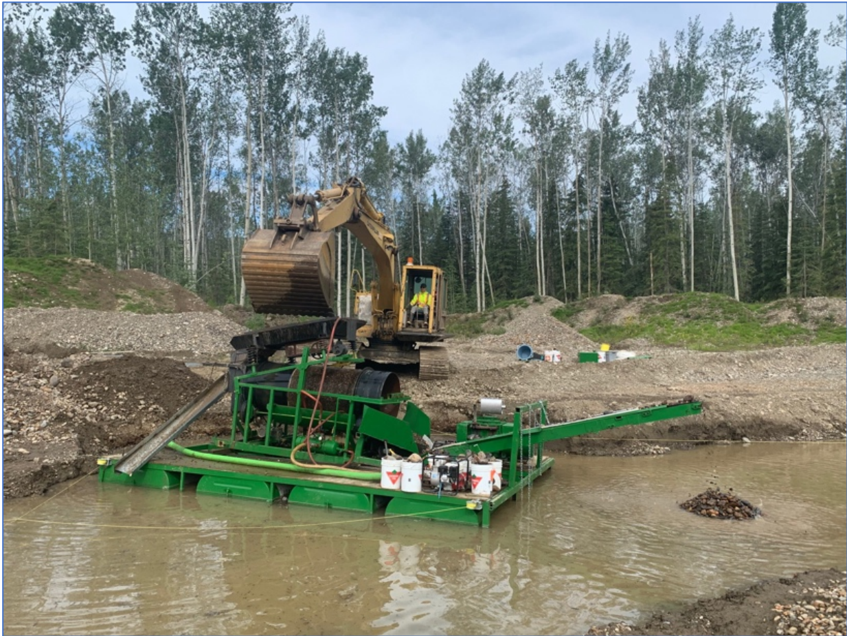
Figure 6. Testing with floating trommel and Dream Mat system
