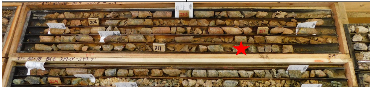
Figure 7-7: Location of TerraSpec reading on DDH 80-18 (218 ft.) and corresponding spectra plot (K-illite signature)
