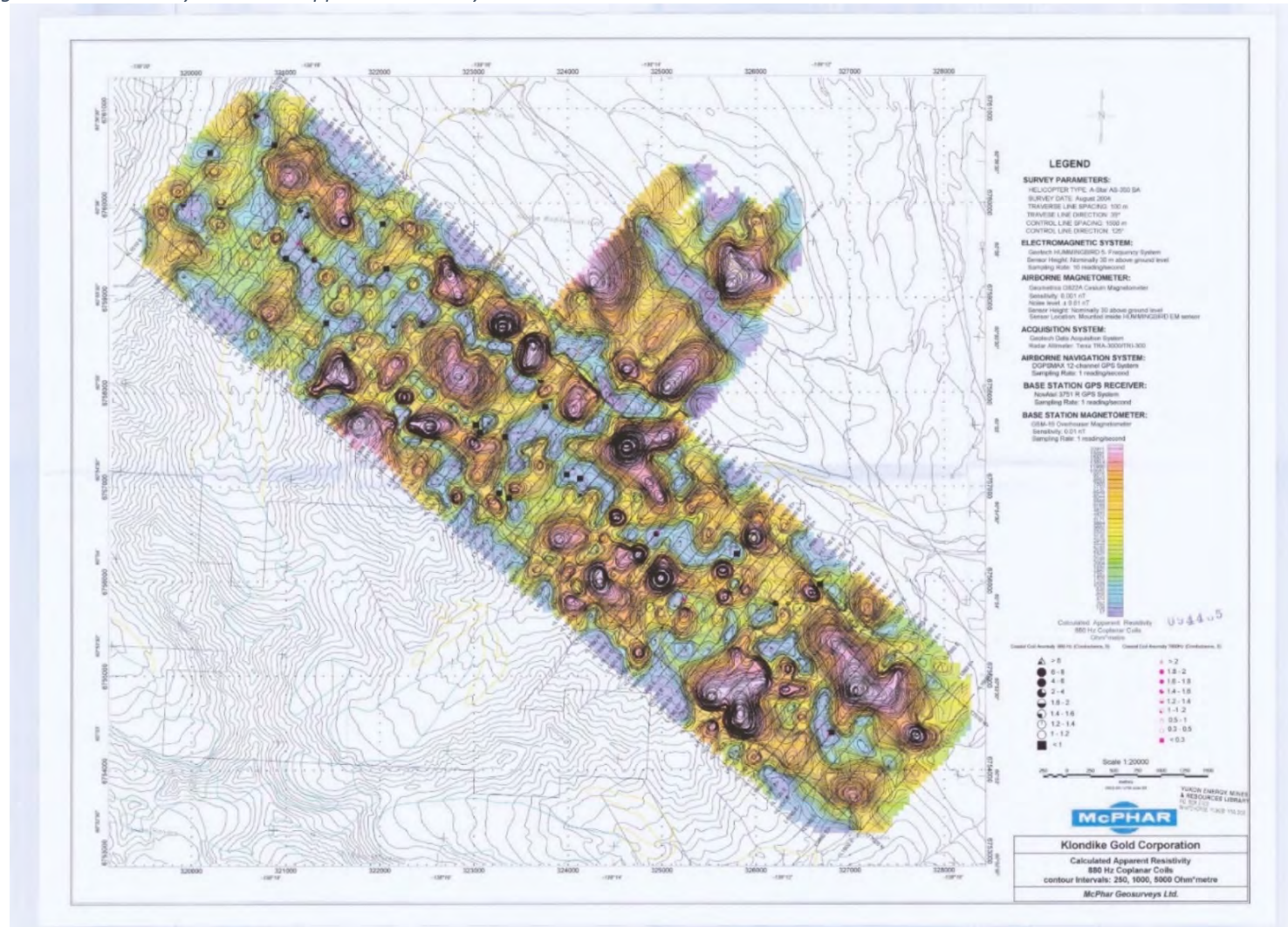
Figure 4: HLEM survey calculated apparent resistivity
