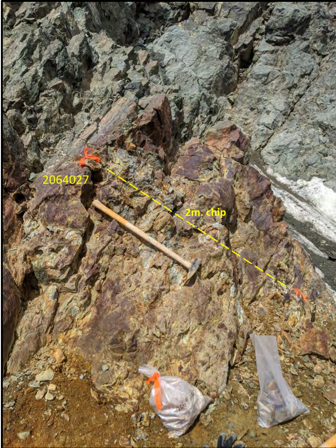
Photo Plate 5: Location of 2 metre chip sample # 2064027. Chip was taken due to the occurrence of massive sulfide bands (pyrite ± chalcopyrite-bornite) within highly gossanous and brecciated, iron-oxidized, mafic volcanic rocks (basalts). Pillows evident. Chip sample taken 25m. from main Telluride massive sulfide showing. Sample bag 2064026 (also pictured) was taken at another location just down-slope from this location (see Figure 33, page 74).
