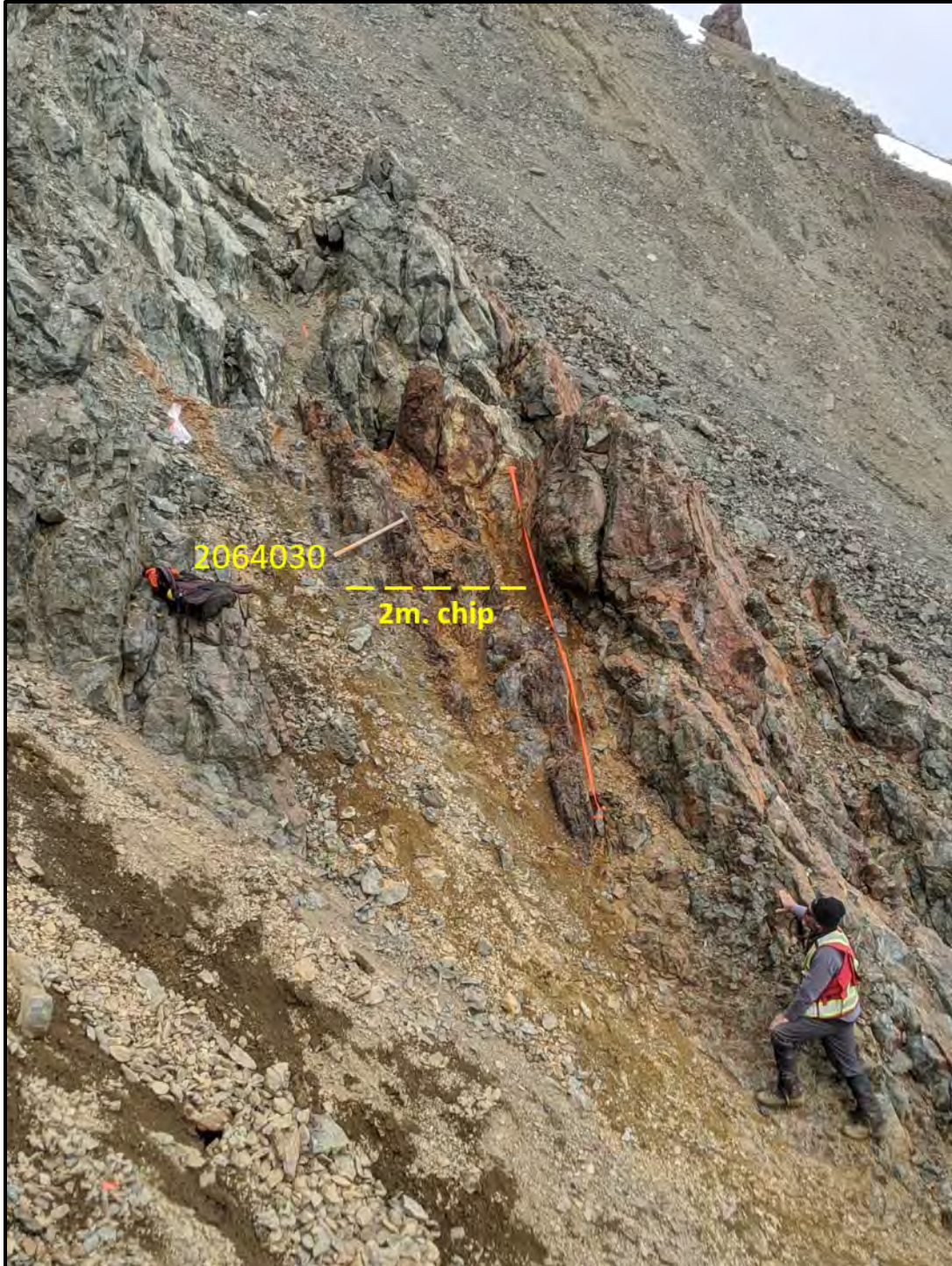
Figure 35: Nearly vertically-dipping, south-facing massive sulfide lens of the Telluride showing. Located 10m away and along strike from the north-facing outcrop (photograph taken standing on the north-facing outcrop). A 2m, massive sulfide lens hosted within Fe-oxidized, sheared mafic volcanics (basalts) with evident pillow structures.
