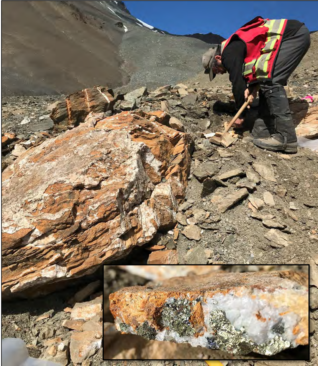
Photo Plate 7: Boulder source of samples 2064215 and 2064215. Quartz-carbonate stockwork veining hosts clots of chalcopyrite, galena and minor sphalerite. Sample 2064214 assayed 2.283% copper, 1.760% lead, 1618 ppm zinc and 40.5 ppm silver. Sample 2064215 assayed 2.471% copper, 7188 ppm lead, 1396 ppm zinc and 26.9 ppm silver.
