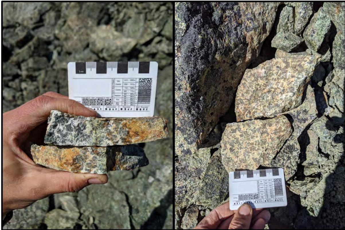
Photo Plate 2: The phaneritic, intermediate volcanic host rock interpreted as a diorite but previously mapped as a gabbro. Minerals include hornblende, augite, plagioclase and/or bleached K-feldspar \pm quartz and biotite. Rock is pervasively propylitic-altered (chlorite and epidote replacing mafic minerals) \pm argillic alteration (clay) of feldspars. Host diorite is cut by quartz-carbonate-epidote-bearing veinlets (mm- to cm-scale).
