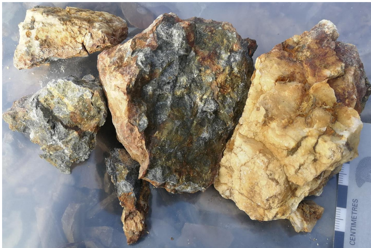
Photo 7 - Float sample ER2034. Quartz cobble found near fault trace with 1-2 cm thick, arsenopyrite-rich vein margin. Minor sericitic alteration on one edge. Sample retrieved below presumed trace of West Fourteen thrust, 34.2 g/t (1.1 oz/ton) Au.
