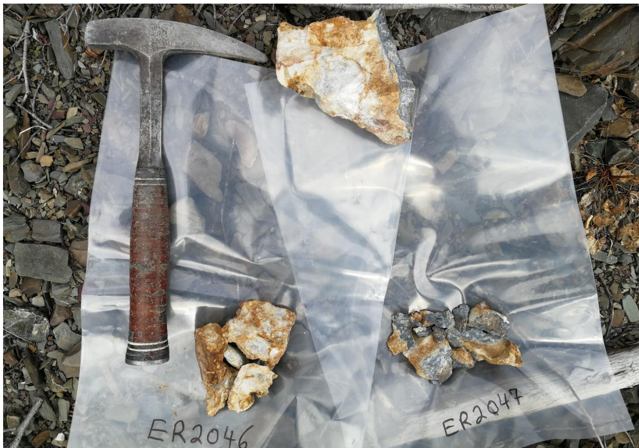
Photo 8 – Vein and vein margin samples crudely split from a float cobble at Avalanche Creek. Vein material sample ER2046, which contained zones of disseminated, submillimeter scale arsenopyrite laths (see photo 6), returned 3.85 g/t Au. Margin sample ER2047, estimated on site to contain roughly 50% arsenopyrite-rich margin and 50% quartz vein material, assayed 21.0 g/t Au. Given the assay for ER2047, and assuming similar grades to ER2046 in the 50% quartz vein material included in ER2047, this suggests a gold concentration in the 1-2 centimeter thick vein margin of roughly 38 g/t Au.
