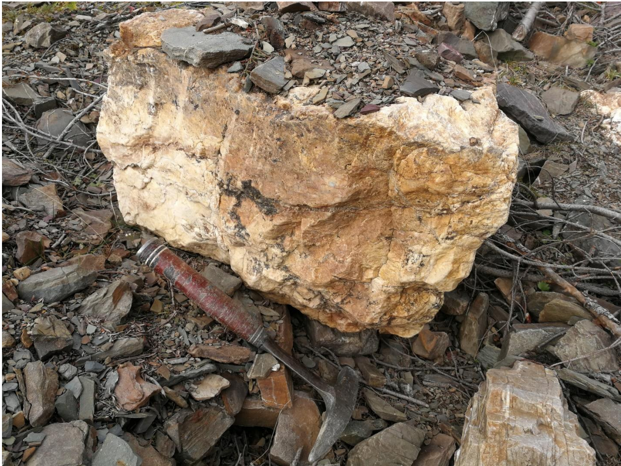
Photo 2 – Mineralized quartz boulder in the Avalanche Creek drainage. Sample ER2045, sampled in 2020, assayed 4.39 g/t Au.
