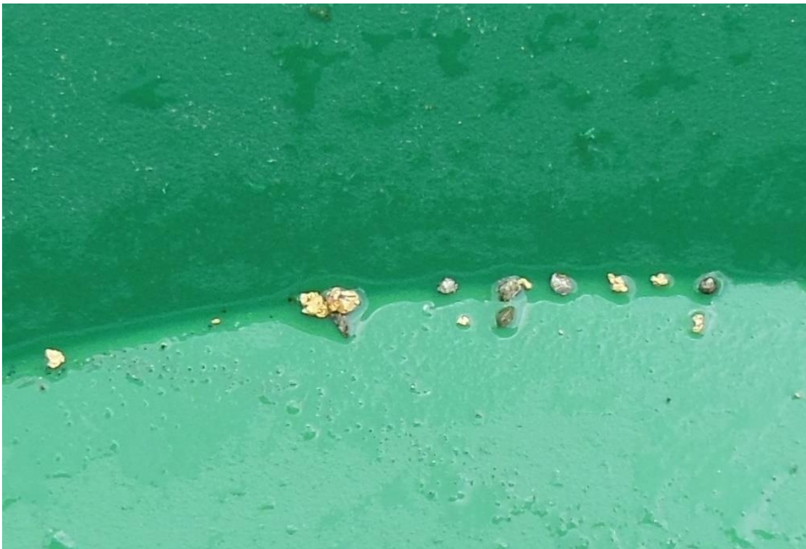
Figure 4 - Sample PATT15-3 from test pit PATTON 2015-01 contained coarse to medium sized hackly gold grains as well as magnetite and rutile.
