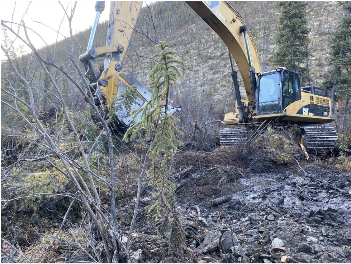
Figure 21 - Test pit 2020-2 was excavated on October 1, 2020 to a depth of approximately 4 metres near auger drill hole 20-7, which had returned 158 mg of gold. This pit was thawed, sloughing prevented a clean sample and bedrock was not clearly reached. Heavy minerals were recovered but no gold.
