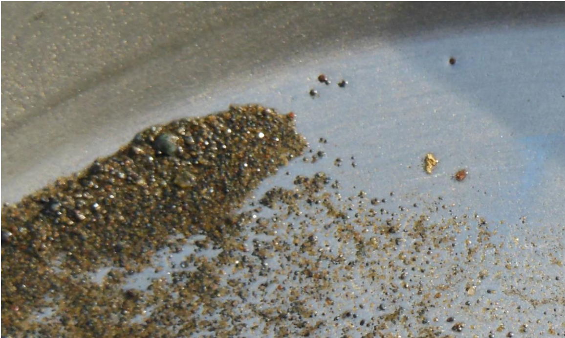
Figure 5 - Sample PATT15-1 was a single pan at the top of the gravel layer in pit PATTON 2015-01. A hackly coarse gold grain and several small colours were recovered along with abundant crystalline magnetite and garnet.
