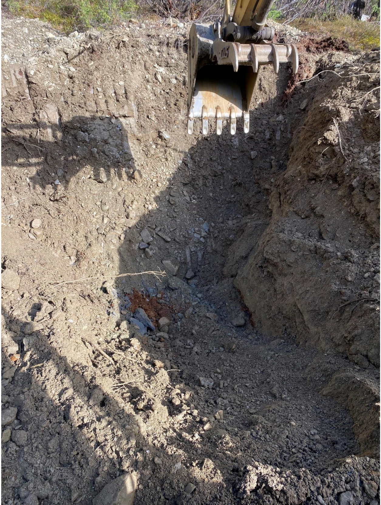
Figure 7: Test Pit #1 with the blue clay and oxidized gravel.
