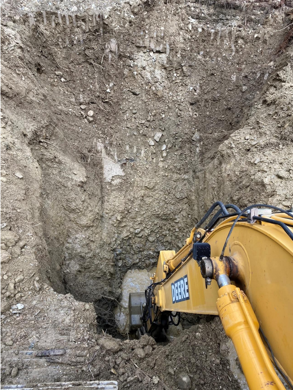
Figure 8: Test Pit #1 with the coarse material layer visible at the bottom of the hole.
