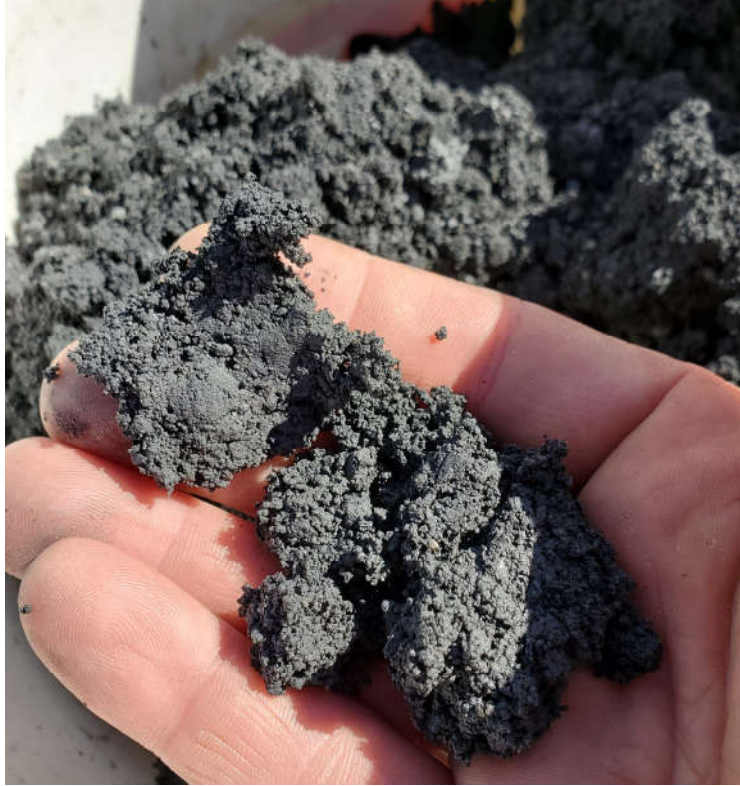
Photo 9: Clay and altered shale at 25 ft in LC-20-009.
