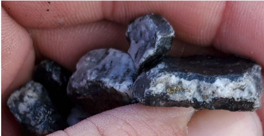
Photo 10: Shale bedrock with quartz-calcite veining and pyrite mineralization in LC-20-009.
