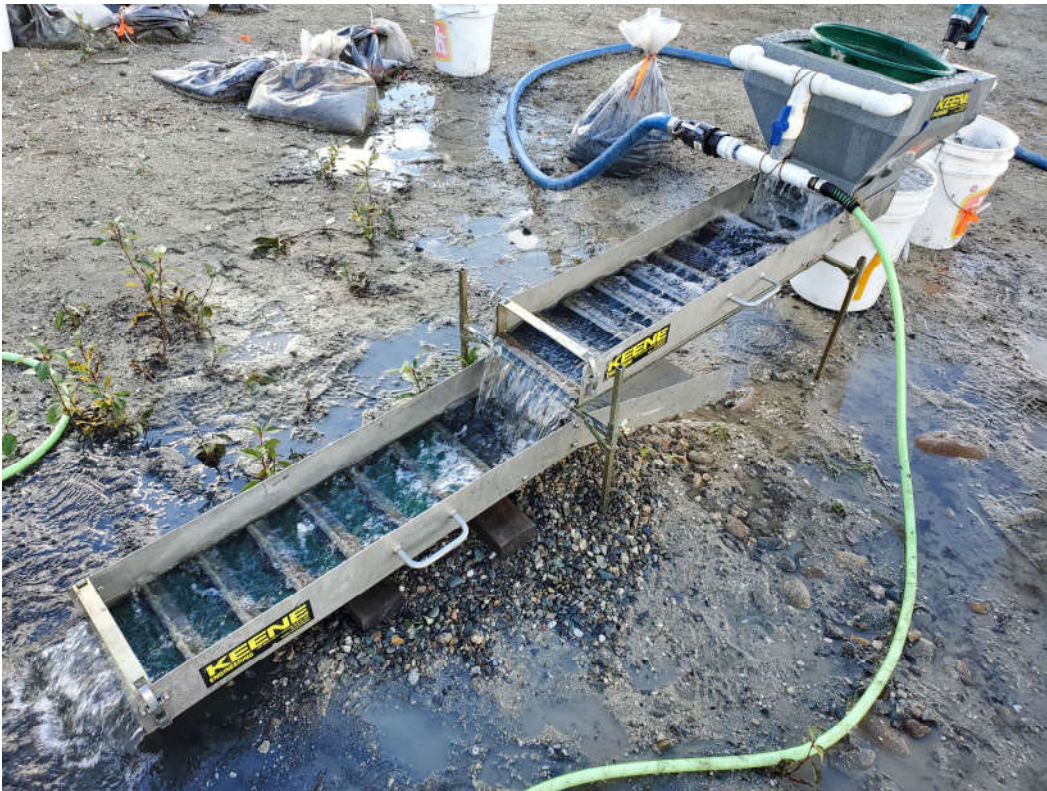
Photo 2: Sluice setup used to process the 2020 drill samples.
