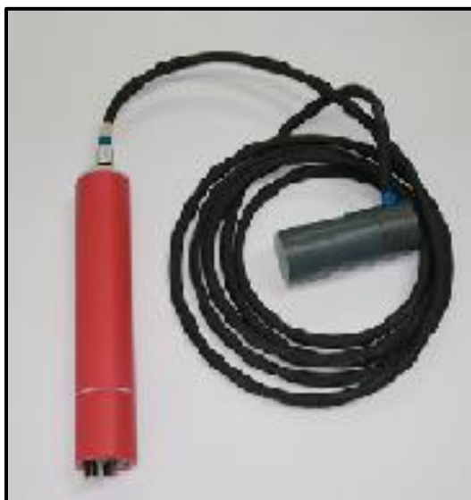
Figure 9: View of CS-3 cesium vapor magnetometer.
