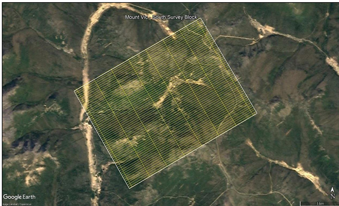
Figure 5: Plan View – Mount Vic - South survey block with actual flight lines in yellow and survey block boundary in white.
