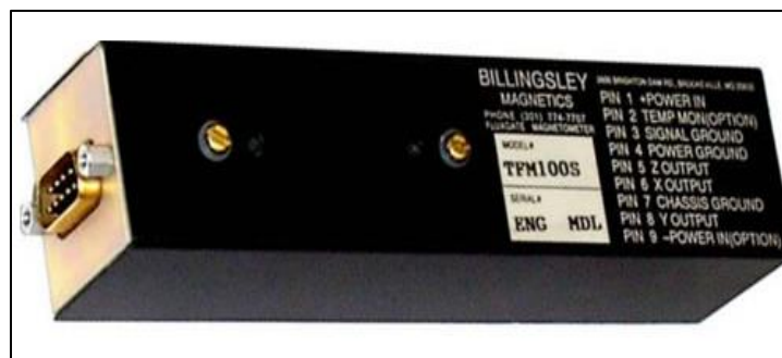
Figure 15: Billingsley Triaxial fluxgate magnetometer.
