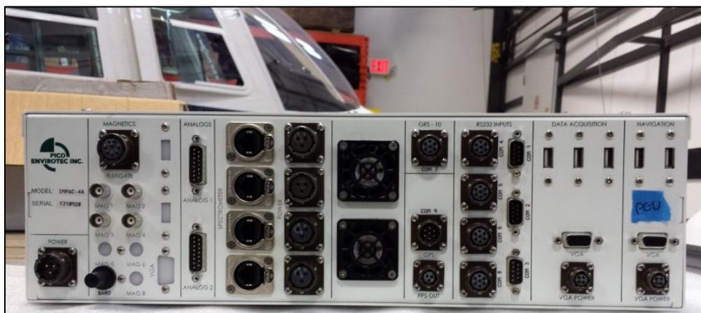
Figure 12: IMPAC data acquisition and navigation system.
