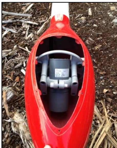
Figure 10: View of "stinger" configuration. Cesium vapor magnetometer sensor orientated 45° from vertical to couple with local magnetic field.
