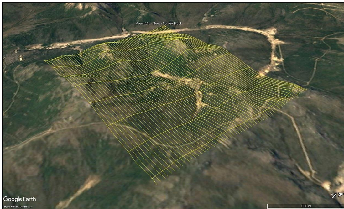
Figure 6: Terrain View – Mount Vic - South survey block with actual flight lines displayed in yellow.
