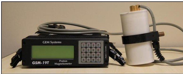
Figure 14: GEM GSM-19T proton precession magnetometer.
