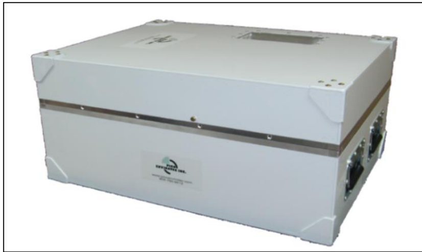
Figure 11: AGRS-5 gamma spectrometer system with five detectors; a total of 21 litres NaI(Tl) synthetic crystals with 4 down and 1 up.
