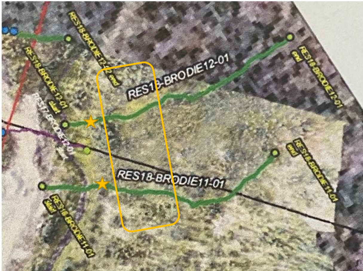
Brodie 11 and 12 Resistivity Lines with Drill Locations and Channel location
