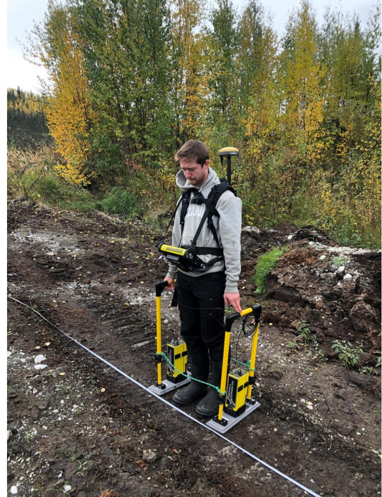
Figure 1: Field survey of 2020 GPR project, left is MALA GX system with 160 MHz shielded antenna, right is PulseEKKO with 200 MHz antenna.
