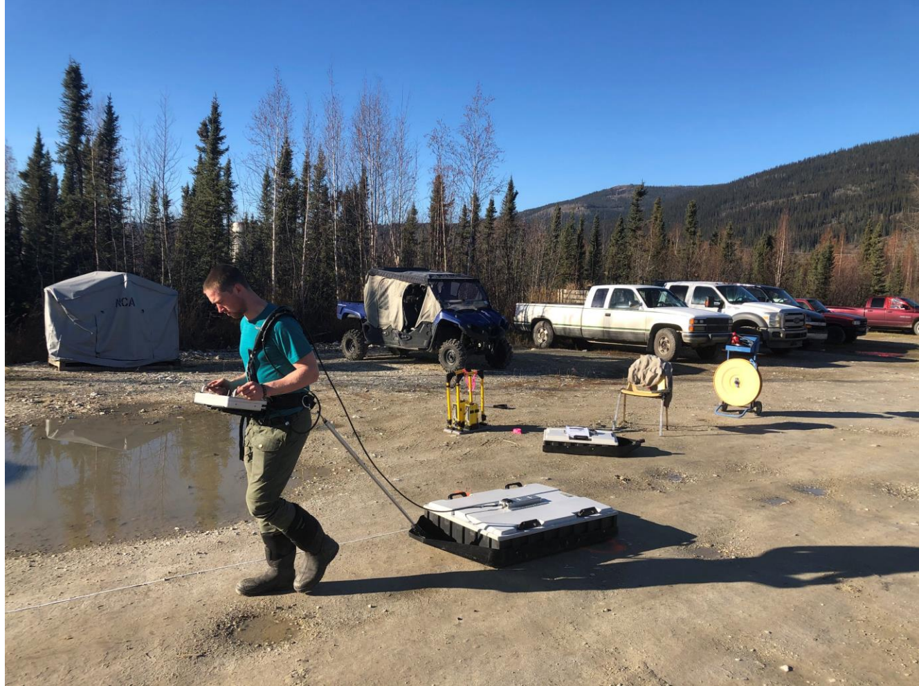
Figure 1: Field survey of 2020 GPR project, left is MALA GX system with 160 MHz shielded antenna, right is PulseEKKO with 200 MHz antenna.
