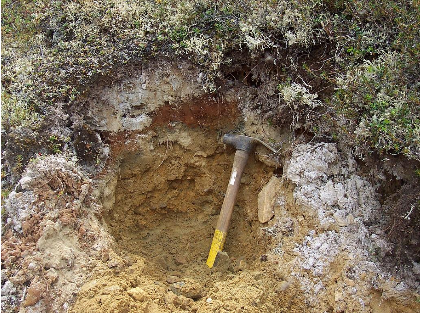
Photo 3. Profile of sand unit SAN at about 2425E/3550N along south bank of Montgomery Creek, showing organic layer, fine sand/ash layer, hematitic oxidized layer, limonitic oxidized layer and unaltered tan-brown coloured sand at bottom.
