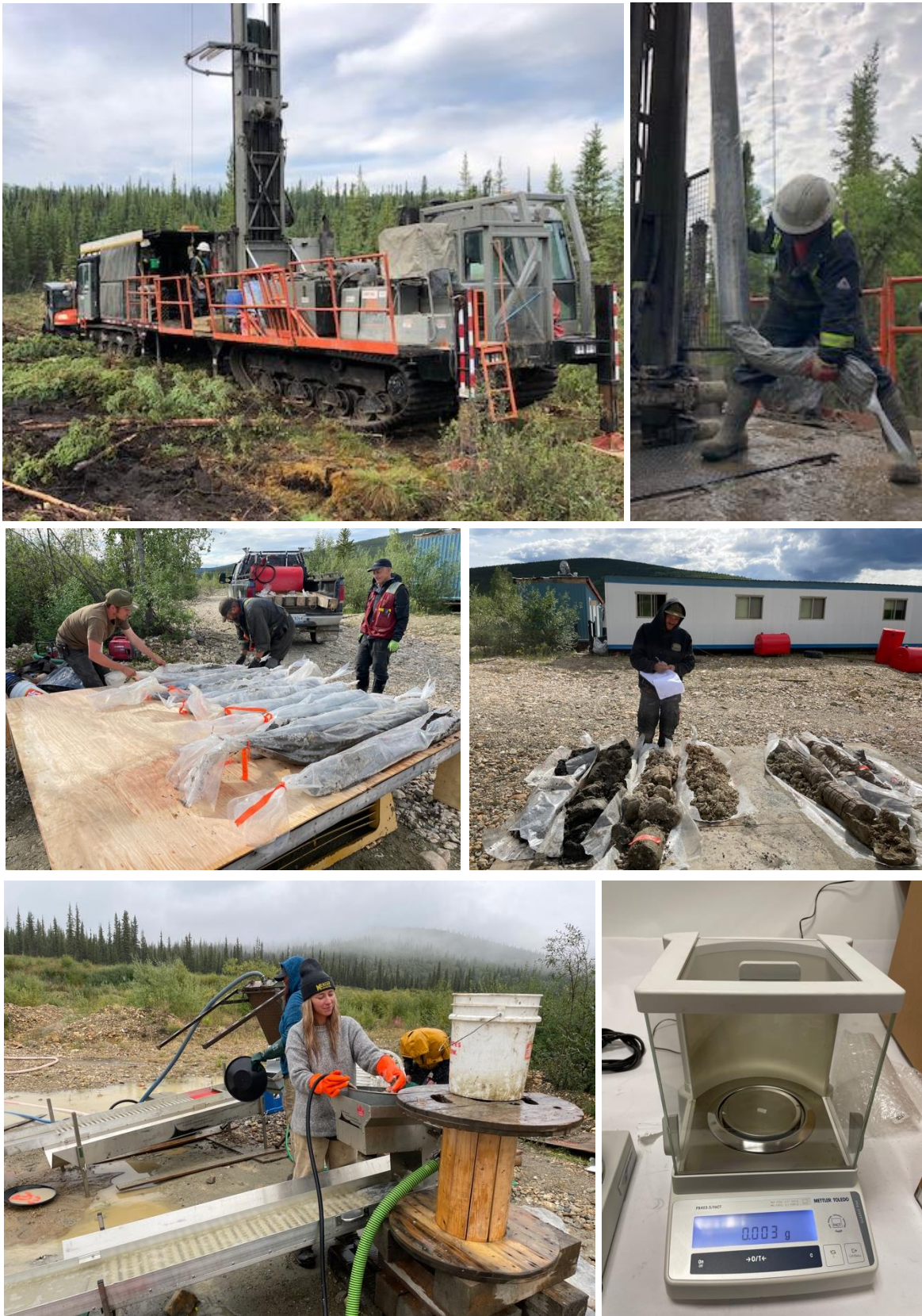
Figure 10 - Photos showing the sonic drill program conducted by Mud Bay Drilling Ltd. The drill was a Boart Longyear LS600 mounted on a Morooka carrier, using 6" casing. The drill was supported by a second tracked vehicle. Samples were logged at the Sulphur Creek camp, and processed using Devin Vortex sluice boxes. The placer gold was weighed using a high precision digital scale.
