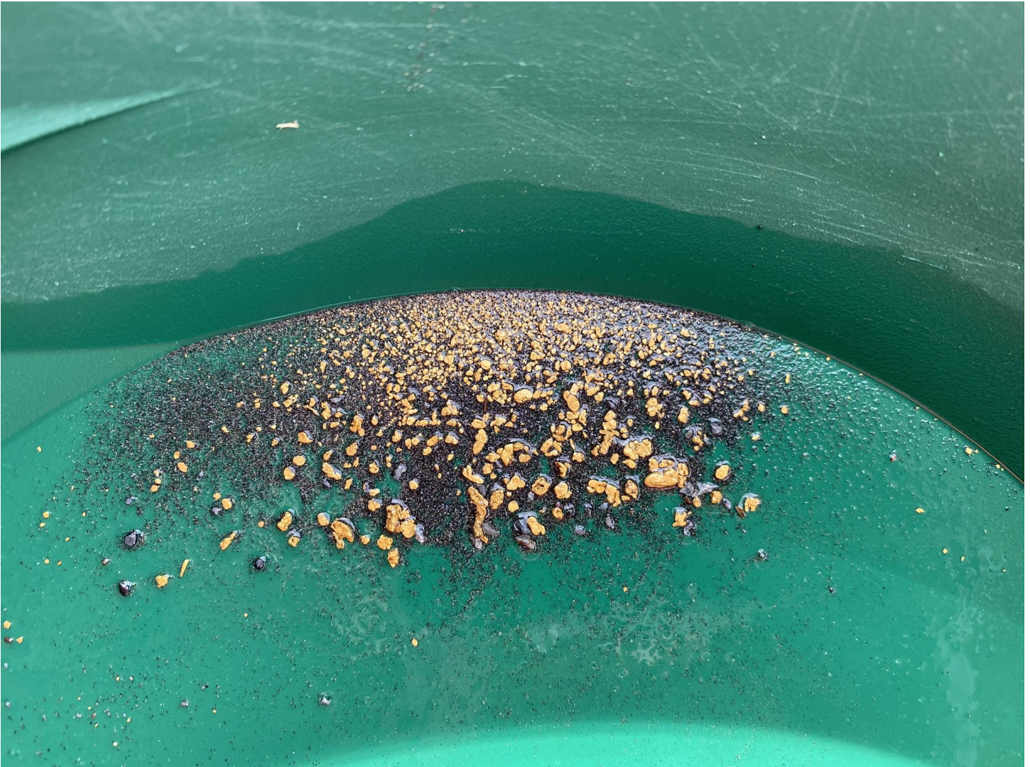
Figure 6 - Placer gold recovered from bulk sample collected near Discovery Outcrop, Australia Creek. The gold weighed 3.25 grams.
