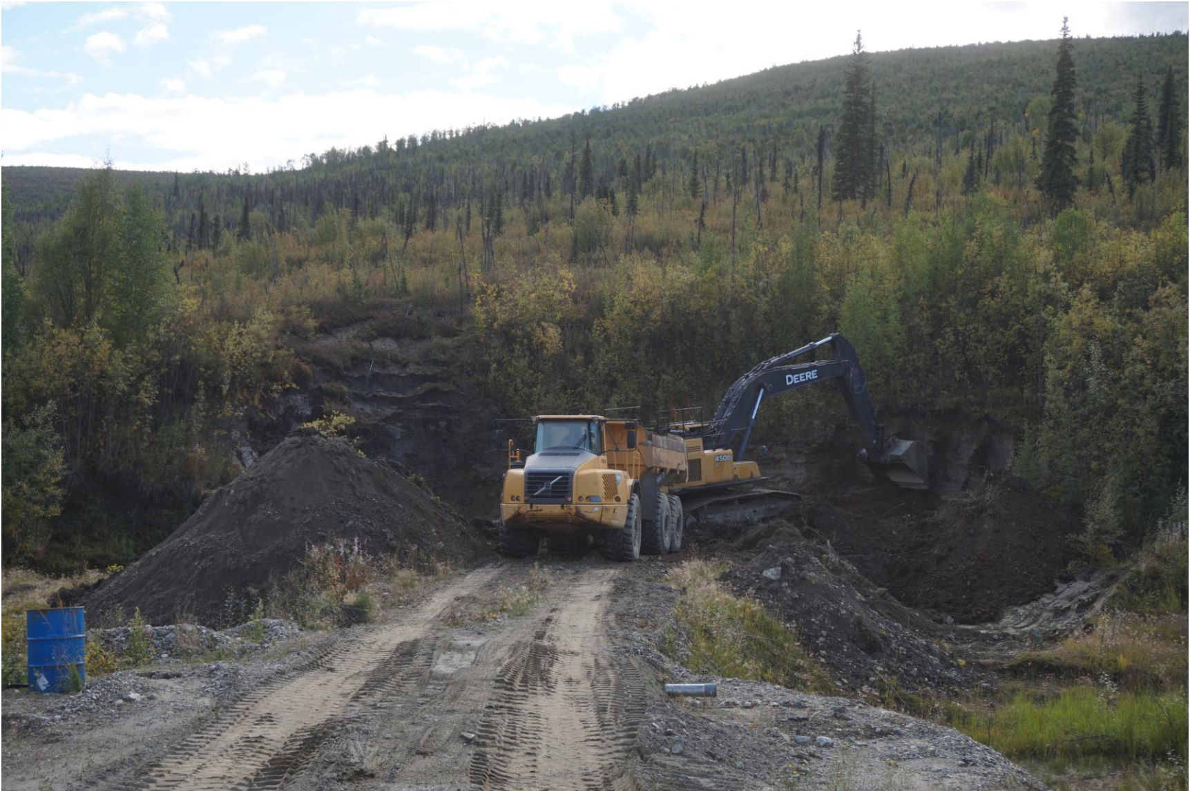
Figure 6 – A 450DLC John Deere excavator loads a 35D Volvo rock truck while bulk sampling in the upper claim block.
