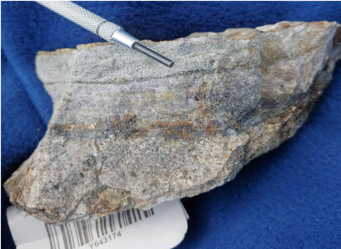
Figure 5: Monzonite float showing parallel bands of magnetite + chalcopyrite in quartz + k-spar veinlets. This sample assayed 0.012 ppm Au, 2.3 ppm Ag, 342 ppm Cu, 591 ppm Pb, and 1085 ppm Zn.
