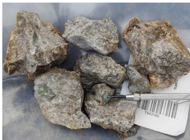
Figure 13: Monzonite float with trace chalcopyrite, malachite, magnetite, and pyrite. Assayed 0.022 ppm Au, 3.1 ppm Ag, 211 ppm Cu, 673 ppm Pb, 907 ppm Zn. Sample Y643165.
