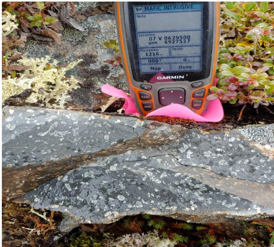
Figure 7: Intermediate volcanic porphyry with fine grained matrix and feldspar phenocrysts
