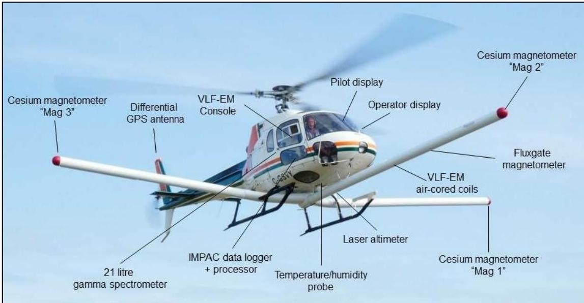
Figure 6: Survey helicopter equipped with three magnetic sensors for gradient magnetic data acquisition, VLF-EM system, and gamma spectrometer.
