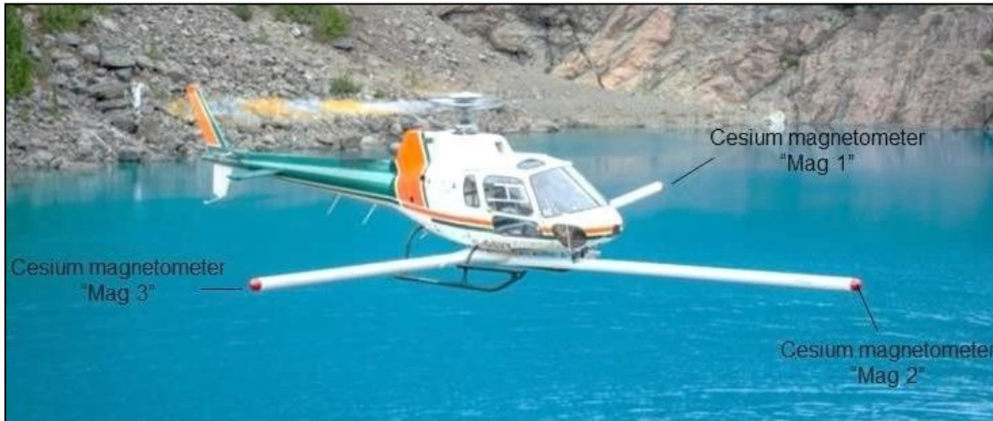
Figure 12: View of triple magnetic boom system.
