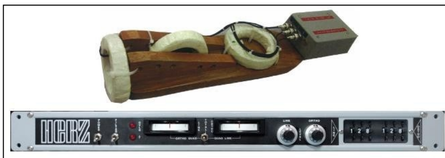
Figure 15: Herz Totem-2A VLF console and sensor (air-cored coils).
