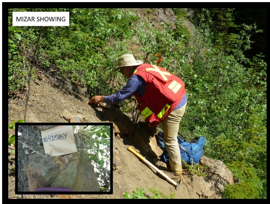
Photo 15: Mizar showing, semi-massive to massive sulphide (095/70) consisting of medium- to coarse-grained sphalerite and tarnished grey minerals thought to be sulfosalt minerals. The showing occurs in the slope of a narrow canyon.
