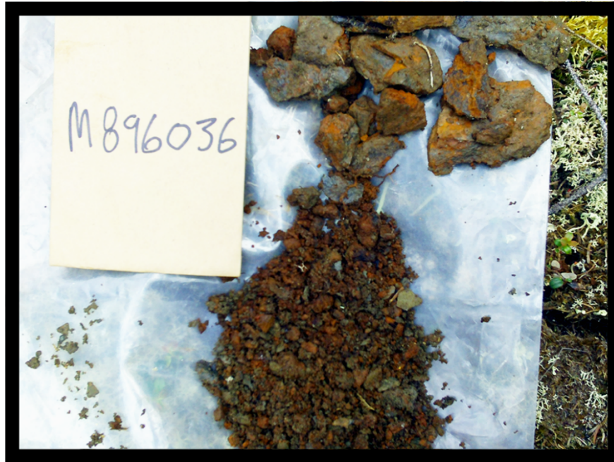
Photo 9: Soil sample M896036 consisting of a mixture of C horizon and glacial till, west of the Nagai Zone. The sample is marked by a dark red staining and abundant rusty fragments. In the soil pit, the rocks show moderate to strong oxidation. Assay returned 196 ppm Zn and anomalous Cu, Pb, and As.
