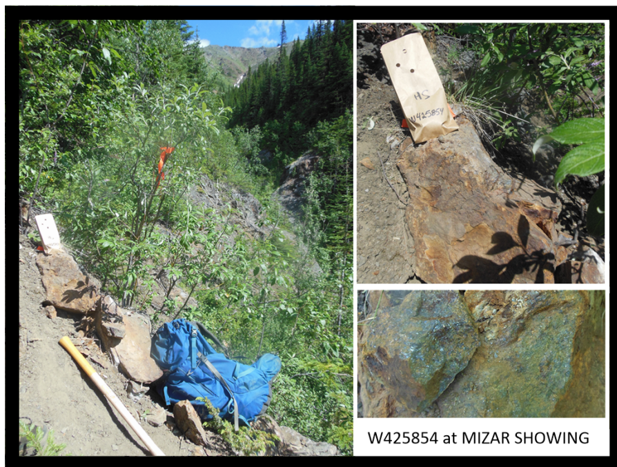
Photo 16: Rock sample W425854 at the Mizar showing, 1 x 0.5 x 0.5m. Host rock consists of dirty limestone/marble and limy siltstone. Bedrock is exposed in the canyon and mineralization may be structurally controlled. W425854 returned 0.51 g/t Au, 2490 g/t Ag, 9900 ppm As, 4.71% Zn, 5.92% Pb, 343 ppm Cu, 4460 ppm Bi and 1035 ppm Sb.
