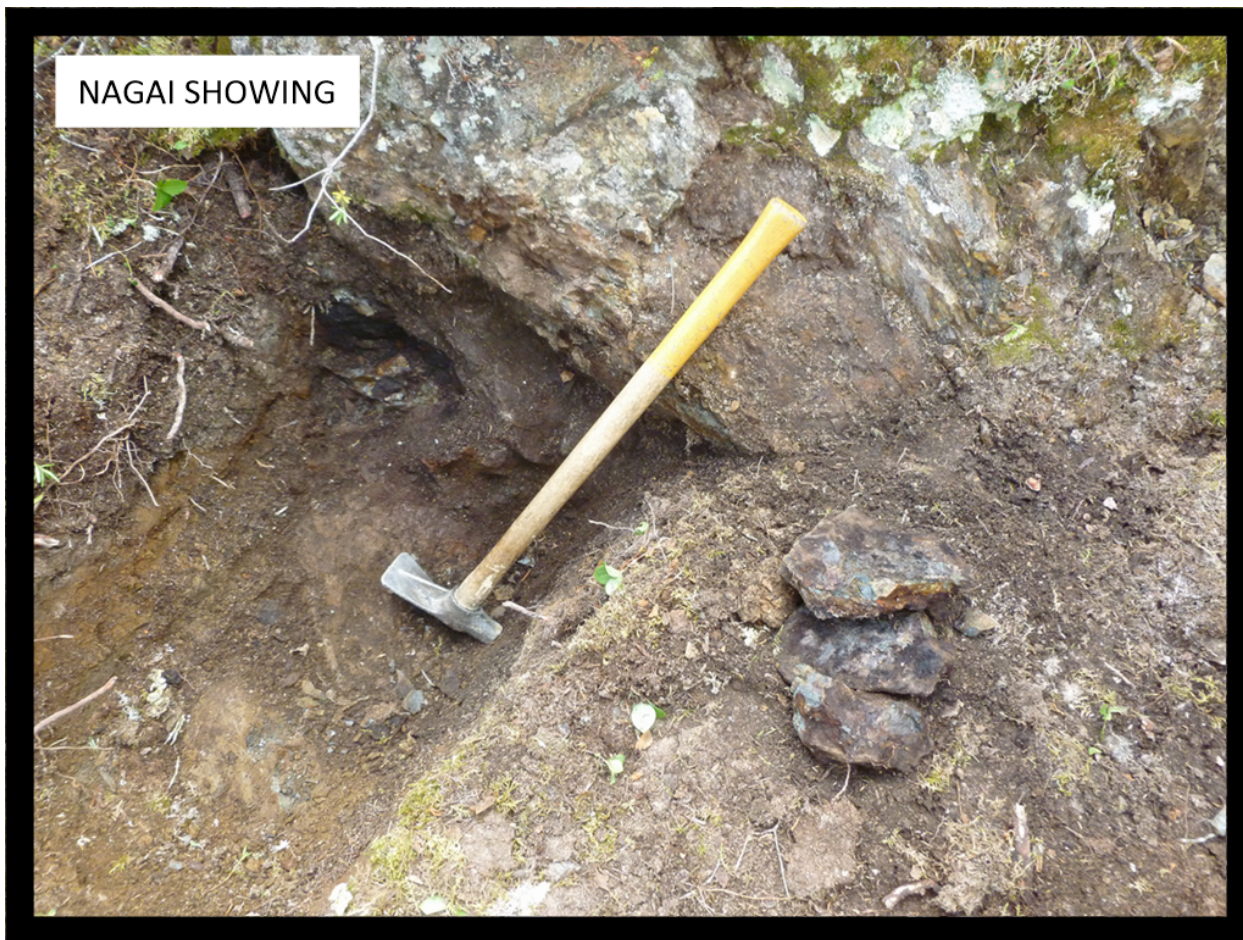
Photo 22: 80 x 40cm hand trench at the Nagai showing. Host rock consists of moderately sheared, chlorite-altered argillite and slaty fine-grained siltstone in the footwall. Abundant disrupted quartz veinlets are associated with pyrite-arsenopyrite-minor pyrrhotite. The outcrop was sampled in 2019. Sample W641858 returned 0.206 g/t Au, 4100 ppm As, trace to negligible base metal content.
