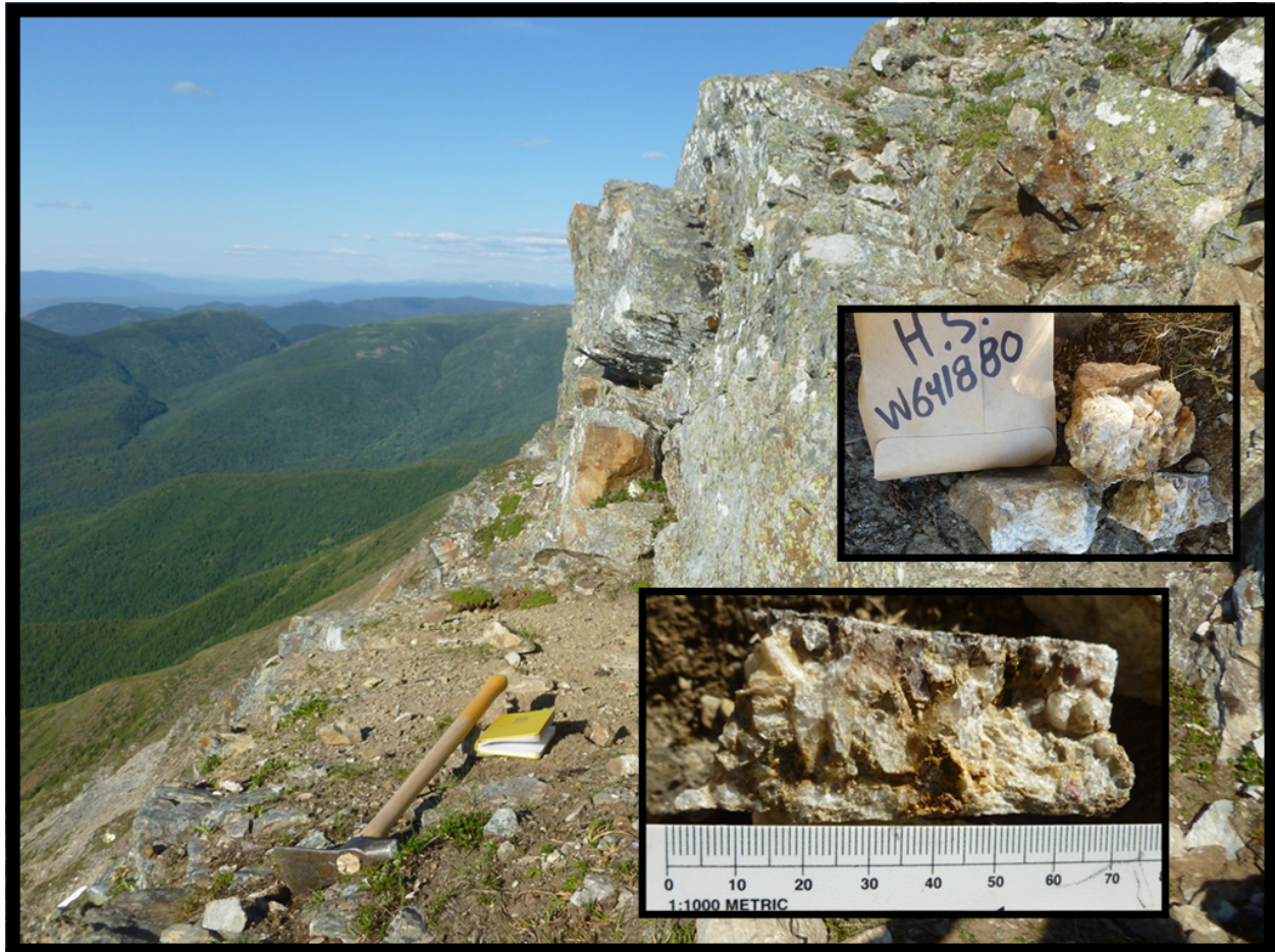
Photo 5: Rock Sample W641880 and sample area: the 2-3 cm wide-coarse crystalline quartz vein is continuous, and it sits on the sub-horizontal surface (316/15) underlying the field book. The vein is weakly mineralized with pyrite-unknown tarnished grey sulphide-limonite in fractures, with trace malachite. The host consists of metasediment (quartzite). Sample returned 0.038 g/t Au, 213 g/t Ag, 2020 ppm Cu, 5580 ppm Pb, 1670 ppm Zn, 59 ppm Bi, and 382 ppm Sb.
