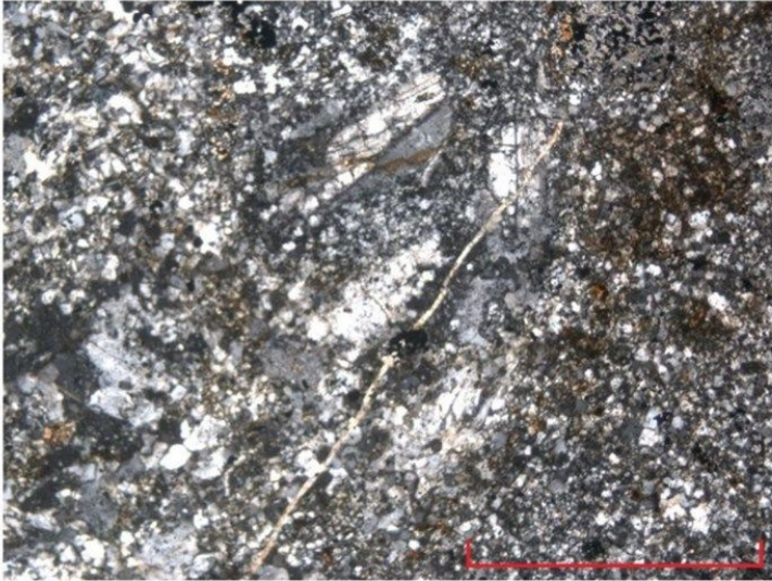
Contact between coarse intrusive and fine-grained volcanic. Crossed polarizers, 1mm scale bar.
