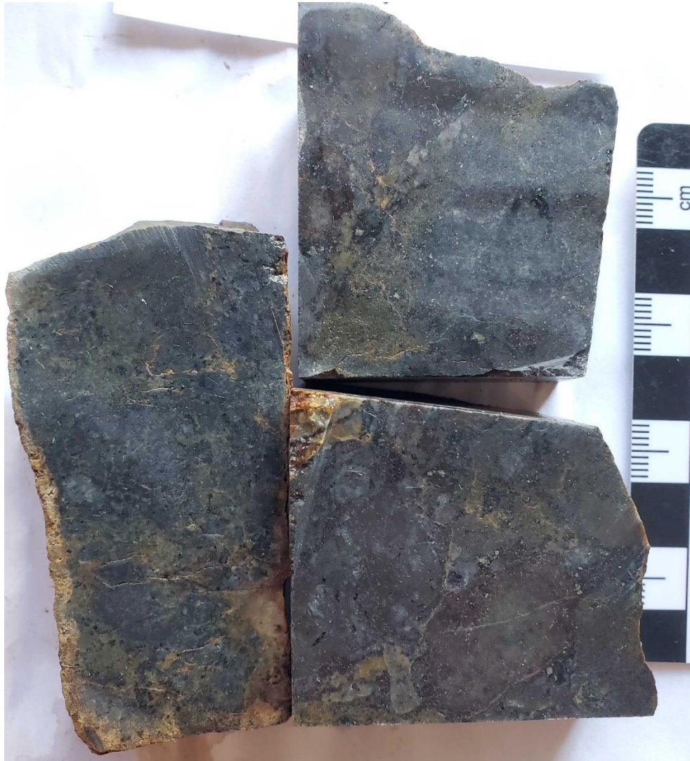
Slabs for P1 – P3. Intrusive- volcanic contact breccia.
