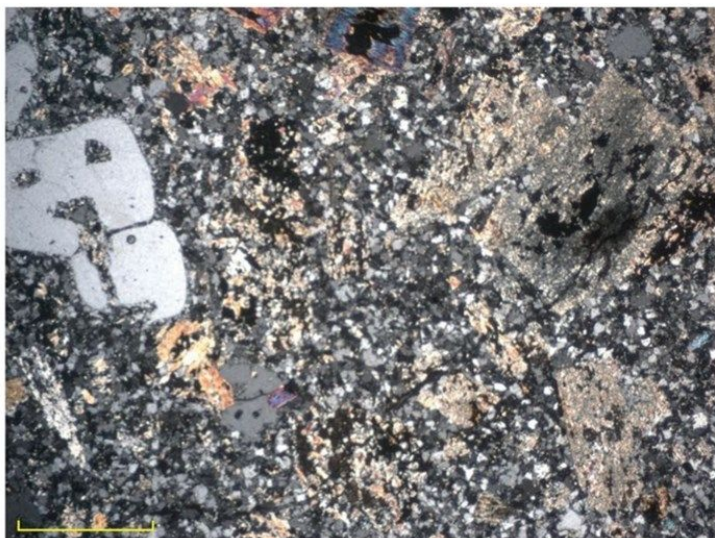
Muscovite, epidote and opaques with altered plagioclase. Crossed polarizers, 1mm scale bar.
