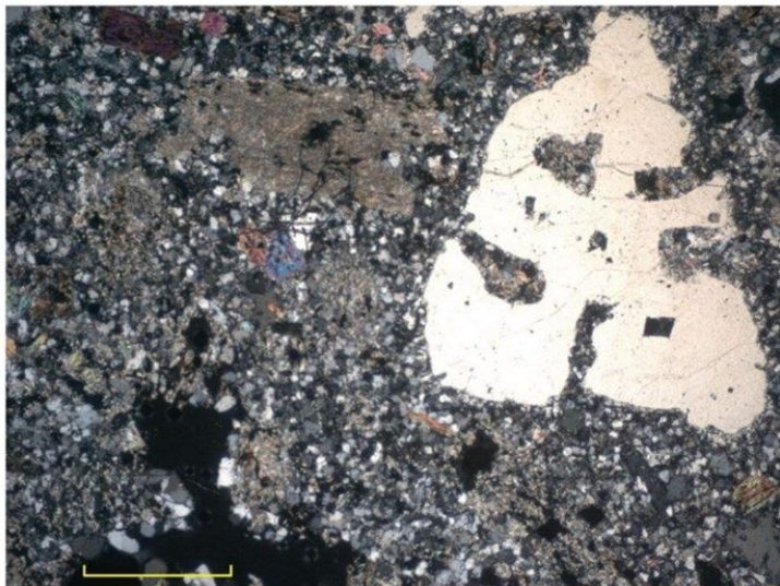
Embayed quartz phenocryst and clay-altered plagioclase. Crossed polarizers, 1mm scale bar.
