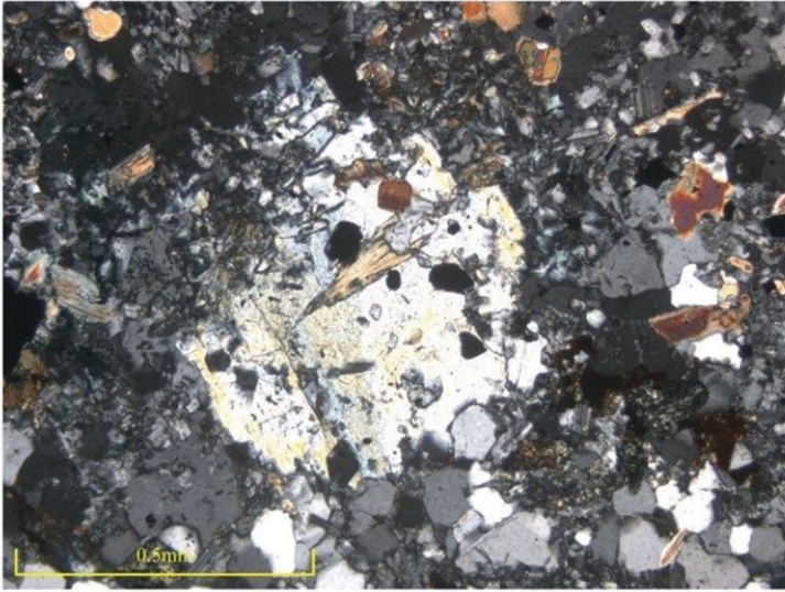
Amphibole included in epidote. Crossed polarizers, 1mm scale bar.
