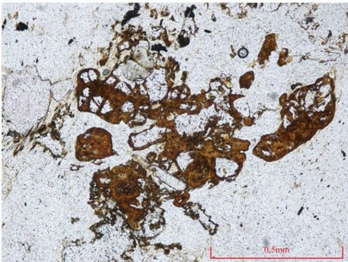
Fe-hydroxides after pyrite. Plane polarized light.
