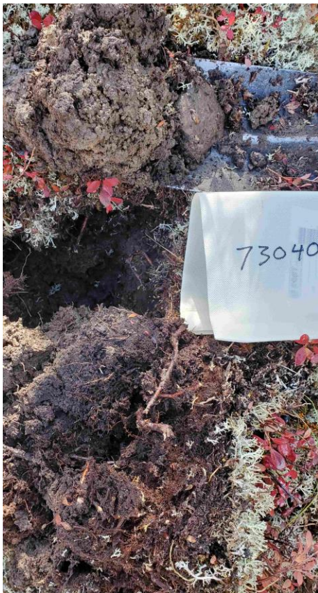
Plate 9. Ah horizon black organic-rich soil above brown B horizon mineral soil. Sample # 5273040.
