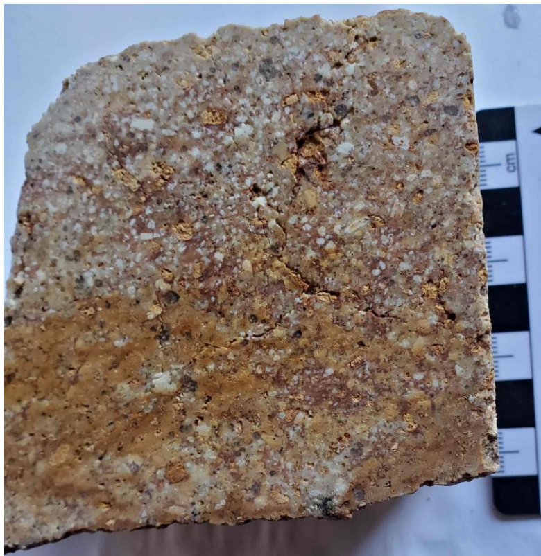
Plate 5. Sixtymile Road pluton, sericite- clay altered.
