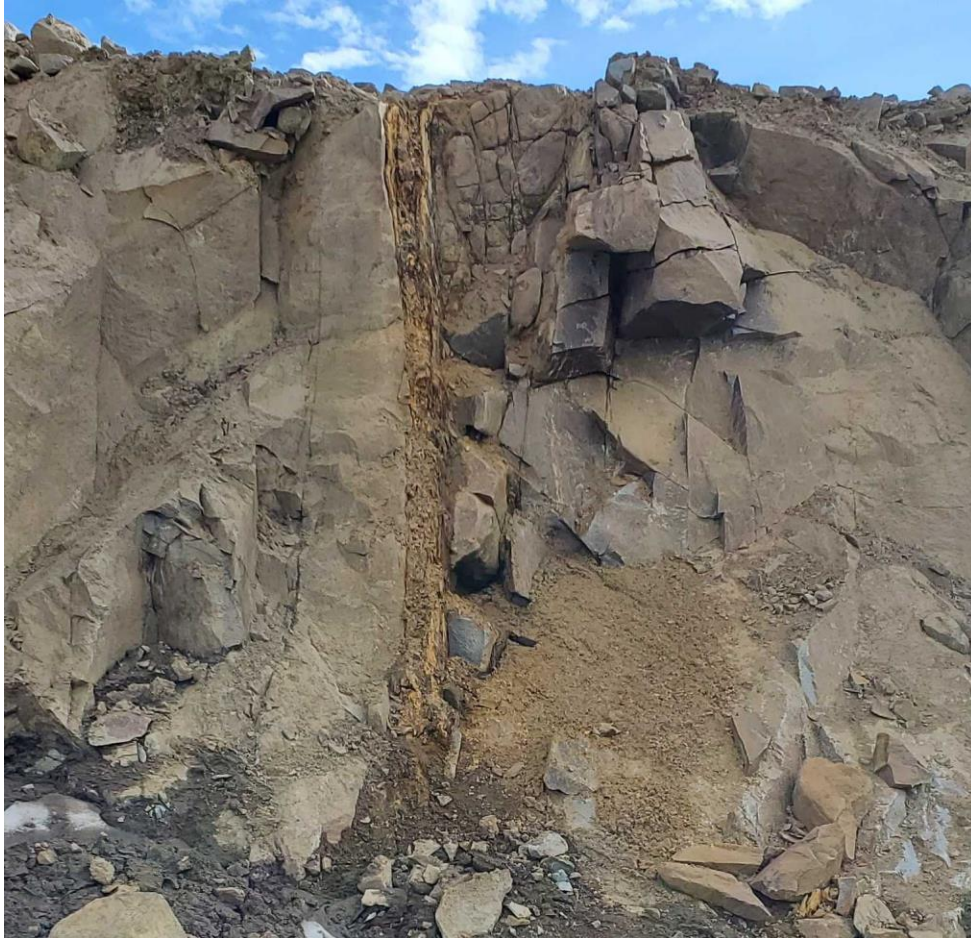
Plate 8. Swede Dome Quarry vein-fault in Prospector Mountain Suite intrusion. Sample # 5285522
