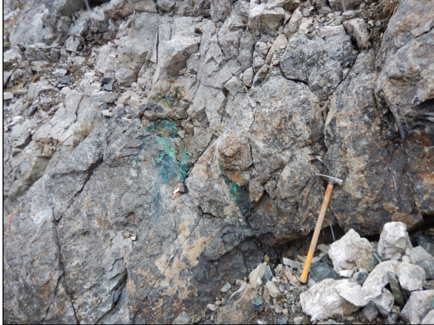
Figure 10: Fracture-controlled and replacement-style arsenopyrite - bornite - chalcopyrite occurrence
