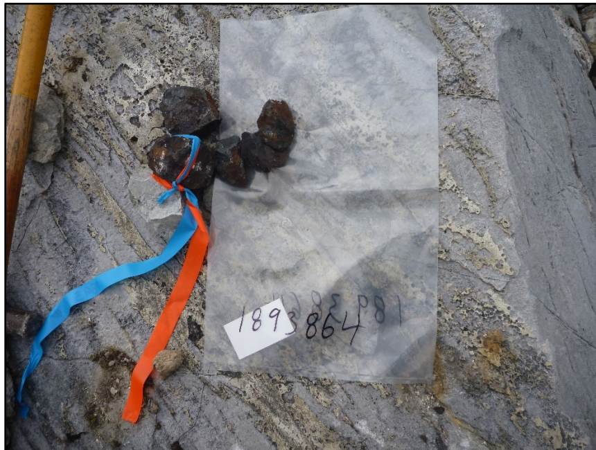
Figure 11: Sample 1893864: Massive magnetite-pyrrhotite-chalcopyrite skarn
