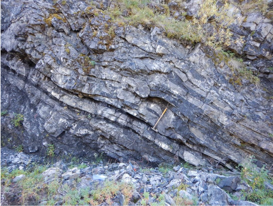
Figure 26. Interbedded grey limestone (limy shale), black calcareous shale (e.g.at hammer head) and black chert (e.g. above end of hammer handle) at sample site RM 405 within the Road River Group unit CDR4 about 900 m east of the Road River Group – Canol Formation contact. View to south from 442549E, 7410014N (UTM, NAD 83, Zone 8W). Hammer handle is about 70 cm long.
