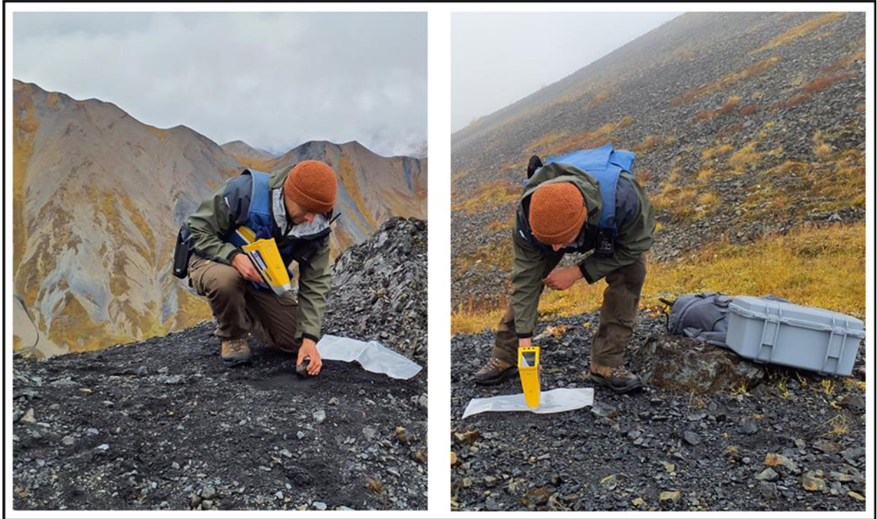
Photo 3: Scott Berdahl operating the XRF portable analyzer. Left picture illustrate a measurement on solid rock, right picture illustrate measurement on compacted "crumbly" black shale. The XRF measurements were repetitively proceeded in-situ on compacted soil/coarse fraction and solid rock at the sample geo-location.
