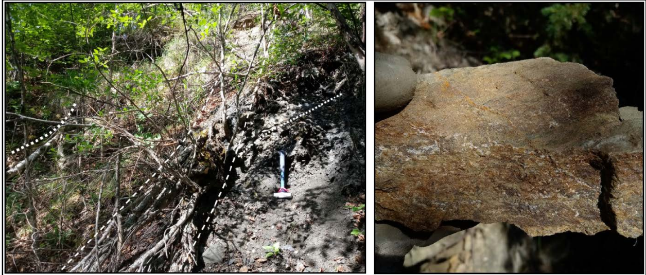
Figure 14: Left: Drag Folding of S2 foliation (Dotted lines) Along Side Fault (Dashed Lines). Right: Graphitic Quartz Vein from Fault (Sample WGO-NM-064).
