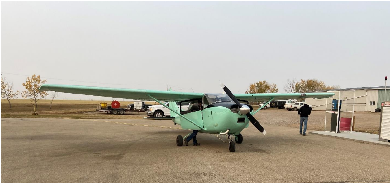
Figure 1: Cessna 182 with MATRIX LiDAR System
