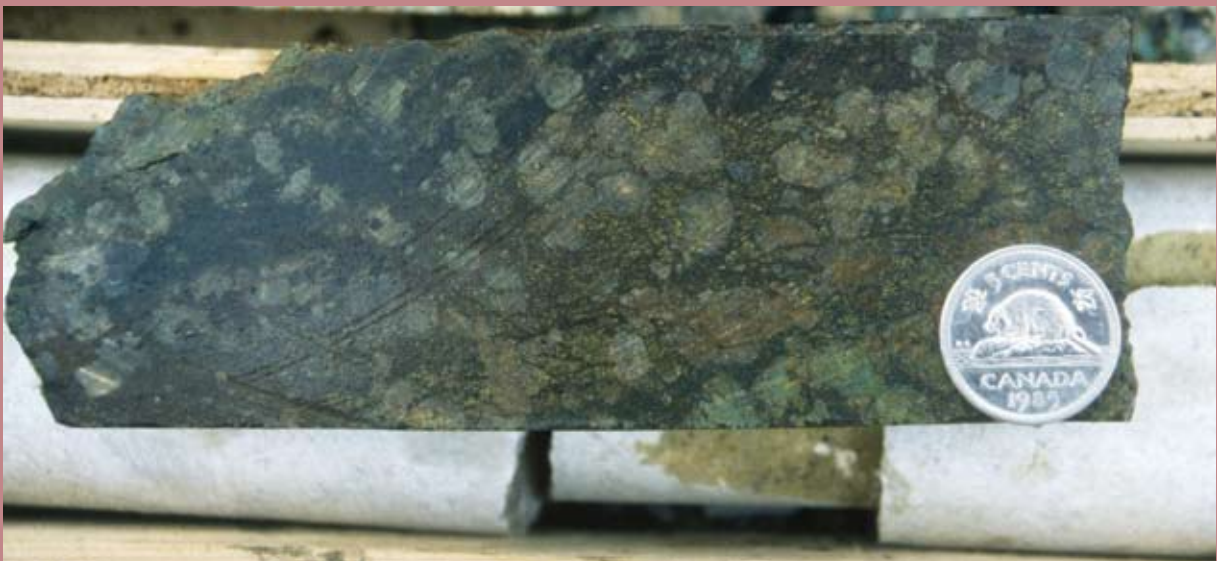
Magnetite, garnet, chalcopyrite and bornite in core from a new copper skarn discovery, the Hat claims, near the past producing War Eagle deposit in the Whitehorse Copper Belt.
