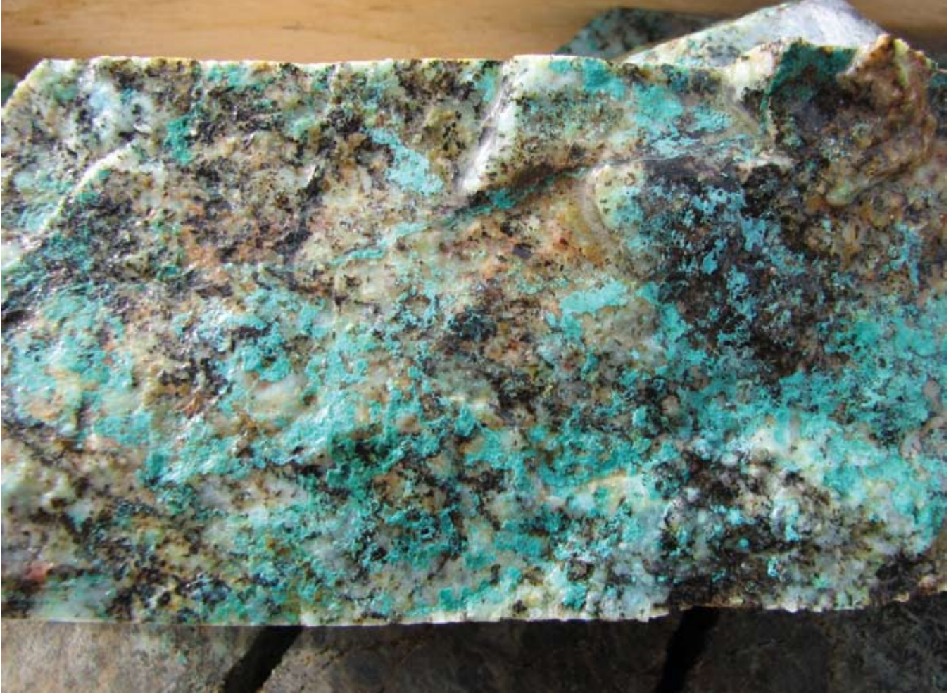
Malachite, a green copper oxide, in drill core from the Williams Creek deposit.
